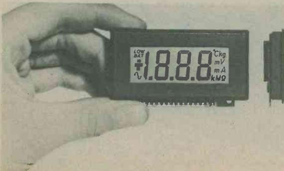
LCD Watch manufacturing techniques are used to reduce the depth to a minimum, the meter being fitted into a DIN bezel of 72mm x 36mm. The 0.6in. (15mm) digits can be read at distances up to ten metres, and the display contains many other useful annunciators. The totally flush face makes it easy to screen print any other logo or engineering unit onto the display.
