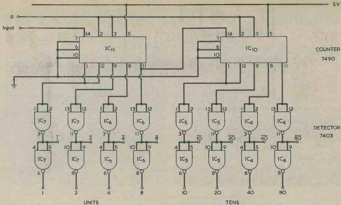
**Fig. 5. Tens and Units counter and NAND gate detector circuits. This section is driven from the 'seconds' output, 'minutes' output or 'hours' output of Fig. 1 via a seconds, minutes or hours selector switch. The outputs of the NAND gates connect directly to the appropriate inputs on the BCD switch.**
