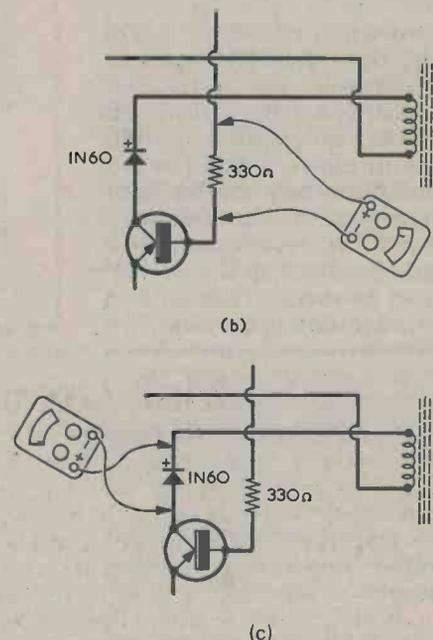
happen to be connected across the one I'm checking. The next things to check are the 1N60 diode and the gated a.g.c. transistor itself. The diode will be the easier, so I'll do that first."
