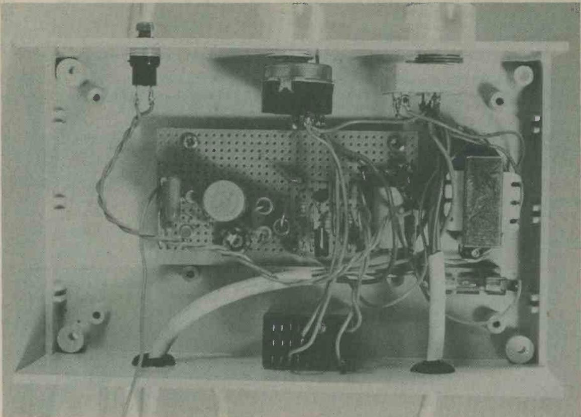
Internal layout inside the case. The mains transformer and fuseholder are positioned at one end of the case. The Veroboard assembly is positioned so that D 1 and D 2, mounted on the board, are close to the transformer. (NB constructors should use 'strain relief' grommets for mains wiring – or at least knot the cable inside the box).
