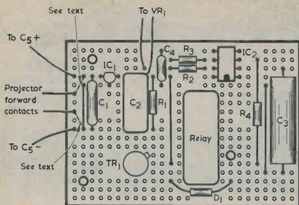
Fig. 3. Component layout on Veroboard
