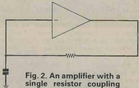
Fig. 2. An amplifier with a single resistor coupling back to an inverting input. A linear amplifier will not oscillate in this circuit, but an amplifier with a Schmitt characteristic will.
