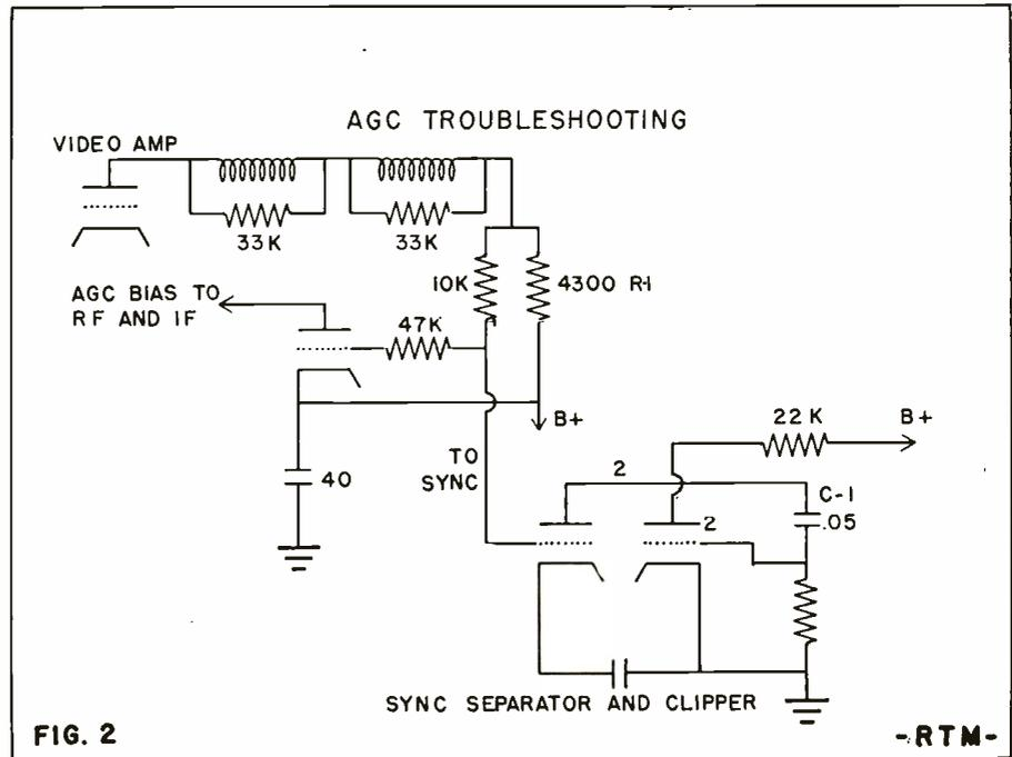
polarity of the signal. Sometimes the signal is DC coupled to the CRT and sometimes it is capacitively coupled. Whenever it is capacitively coupled there must be DC restoration; 3. The synchronization pulses are coupled to the grid of the sync separator tube and fed eventually to the horizontal and vertical oscillators.
