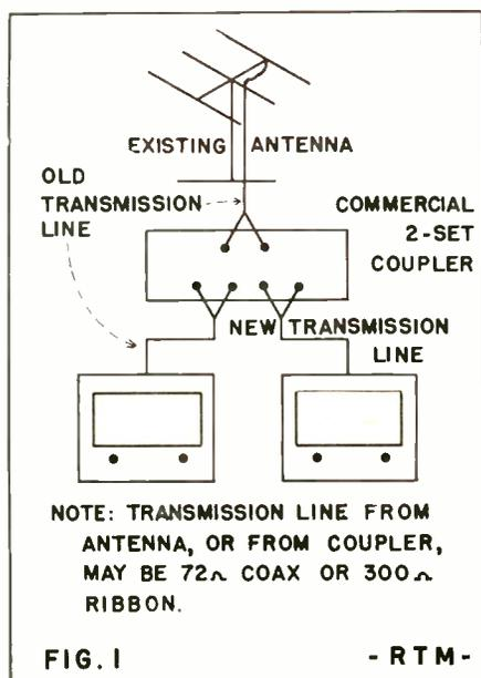
Circuit connections for two-set coupler, connecting FM and TV, or two TV sets, to a common antenna. Coupler is especially useful in apartment house installations or other multiple-dwelling installations.
