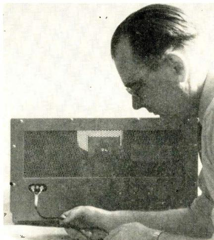
Serviceman cuts quarter-wave stub until interference line disappears from the picture. Stub is a piece of 300-ohm line connected to the antenna input terminals of the receiver; starting lengths, to be used for the various channels on which interference might occur, are shown in Table 1, below.
