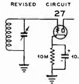
GRID LEAK DETECTOR CONVERTED TO POWER DETECTOR
