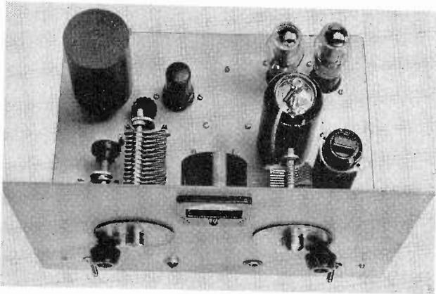
*Another experimental model was built by W6SEM before the final design was constructed. This model is shown to the left. Like the first model, an aluminum chassis was chosen, and the components are again of the conventional receiver-type. A heavy aluminum can was likewise placed over the oscillator coil. Results were entirely satisfactory.*
