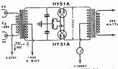
260-watts output can readily be secured from a pair of HY-51A triodes, in the circuit shown.
