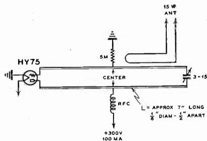
Parallel-wire circuit for 1 $\frac{1}{4}$ -meter operation
