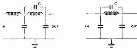
Fig. 7—Showing how by-pass condenser *C* is connected into the circuit, either for choke or condenser-input.
