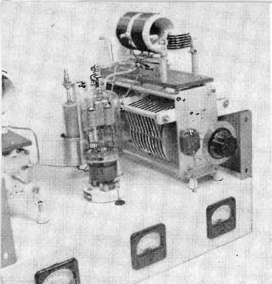
Typical Plate-Modulated R-F Amplifier with new Eimac 152TL triode. E. F. Johnson Inductances with Rotatable Coupling Coils are illustrated. Cathode-Ray Oscilloscope Pickup Coil also is shown.
