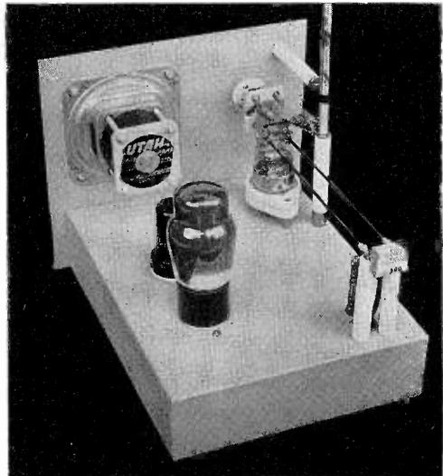
Suitable design for 2 $\frac{1}{2}$ -meter transceiver
