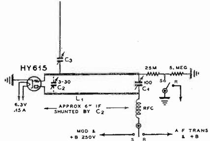
Paralle-wire circuit for 2½-meters therefore, an ideal tube for portables and transceivers.
