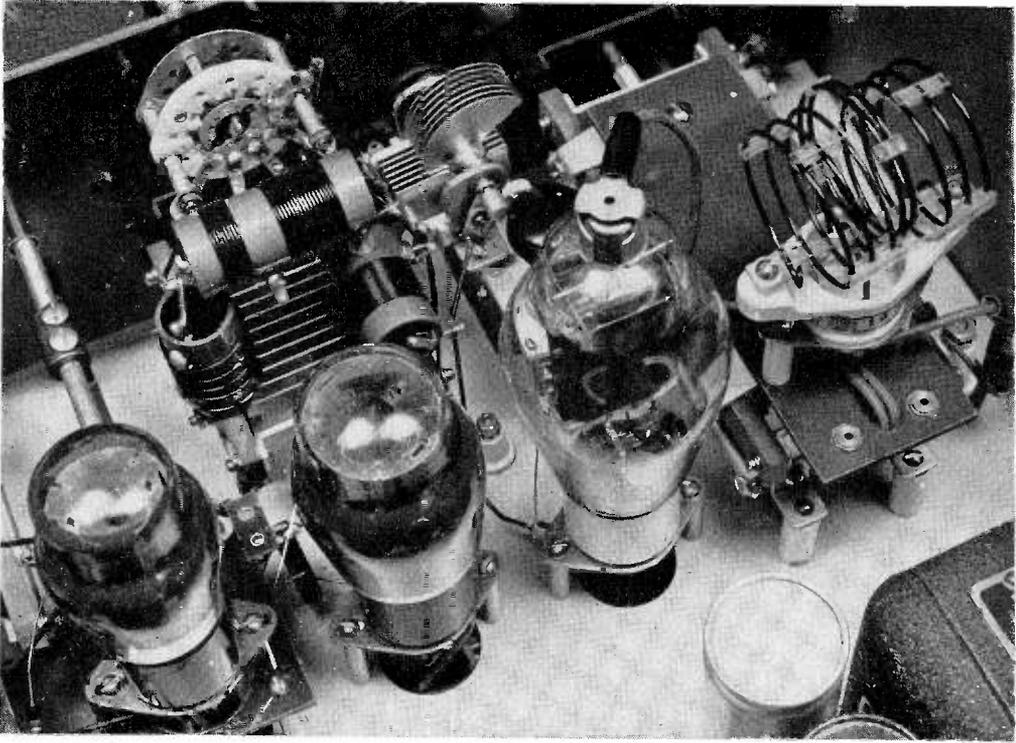
Home-Built Frequency Doubler Stage with Band-Switching and separate coil forms and
