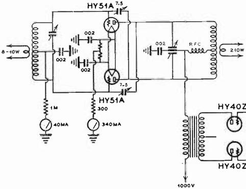
Modulated Amplifier with HY-51As in push-pull. 210-watts output. Only 10-watts drive required.
