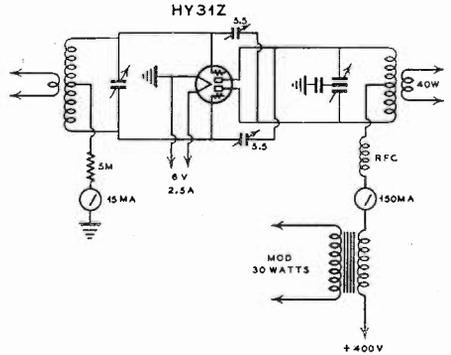
Modulated Amplifier with HY-31Z, 40 watts.
