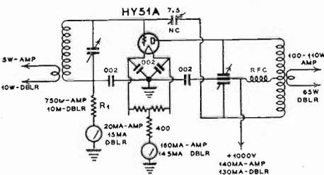
Frequency Doubler or R-F Amplifier with single HY-51A. Doubler output, 65 watts. Amplifier output, 100-110 watts.
