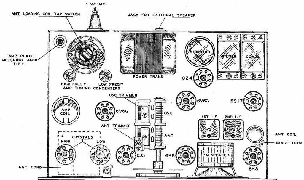
*Parts layout for emergency transmitter-receiver. This diagram will aid the builder in the proper placement of components. Careful thought was given this design, and the prospective constructor is advised to adhere closely to this general arrangement.*
