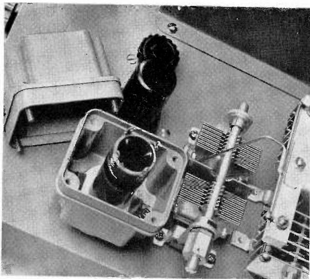
*Looking into the Millen shield can which houses the layer-wound oscillator coil. This coil is wound in three layers, with taps taken according to the data given at the end of the text. The Millen padder condenser is mounted directly alongside the oscillator coil shield. Once adjusted, it is held in position by means of the lock-nut assembly. A small portion of the main tuning condenser is seen at the extreme right.*
