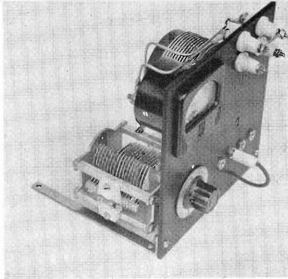
*Versatile Antenna Coupling Unit for Series or Parallel Tuning. Note Plugs and Jacks for Selecting Various Values of Inductance.*
