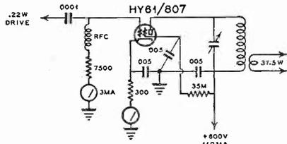
The HY-61/807 Beam Tetrode requires only 0.22-watts drive and delivers 37.5-watts output in the circuit shown.
