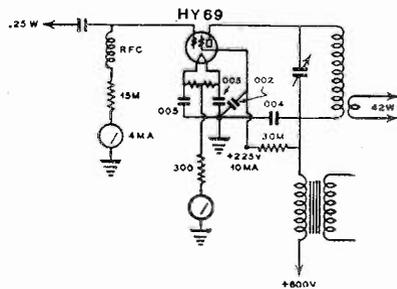
HY-69 Modulated Amplifier, 42-watts output. This tube has a separate lead to the beam plates, brought to a prong on the tube base.
