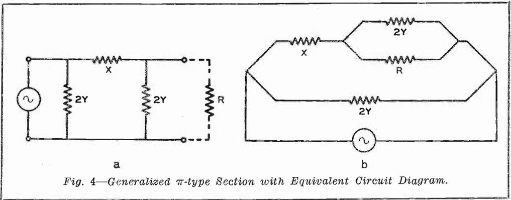
Fig. 4—Generalized  $\pi$ -type Section with Equivalent Circuit Diagram.
