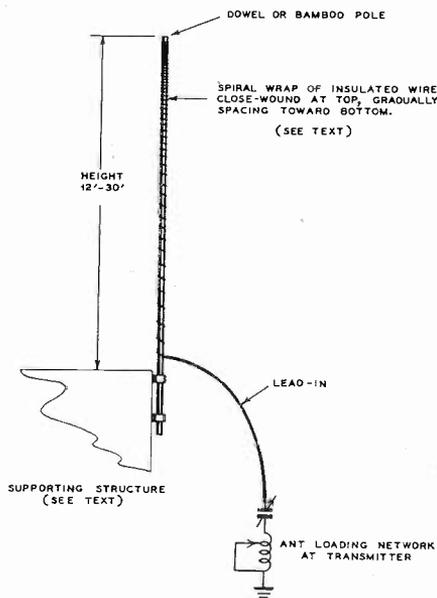
Constructional Details for Portable Antenna.
