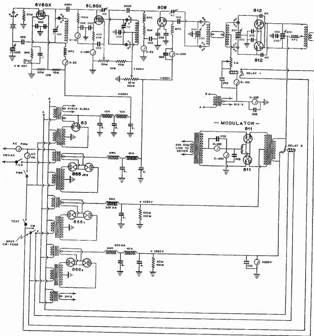
Push-pull RCA-812 transmitter circuit and zero-bias 811 modulator. A popular circuit for the amateur who desired medium-high power output.
