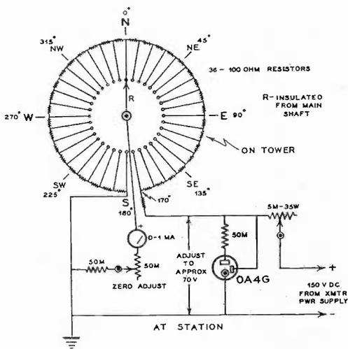
Resistor-box connections for indicating device.
