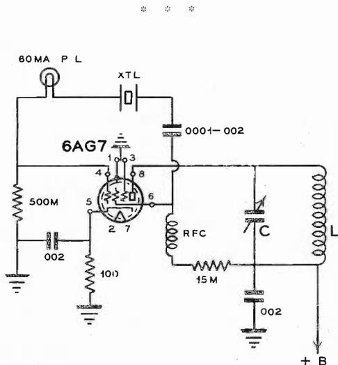
Circuit diagram of Wells Harmonic Oscillator with correct identification for tube pin connections. Many readers report exceptional success from this newest of oscillator circuits. Care must be exercised to select crystals with one "hump" only.
