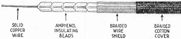
Various items manufactured from low-loss Polystyrene insulating material by the American Phenolic Corporation. Upper view shows details of transmission line. To the right is the Amphenol Polystyrene u.h.f. coil form. Below, left—bead spacers for low-loss lines; right—Amphenol u.h.f. socket, also of Polystyrene.
