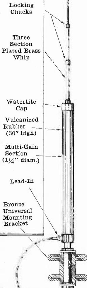
• Here is a practical mechanical and electrical answer to the problem of high gain from short antennas on the intermediate high frequencies. No metal cans, hats or rib structure on the top of the antenna—simply a streamlined vulcanized-in-rubber loading section in combination with a three section whip.
