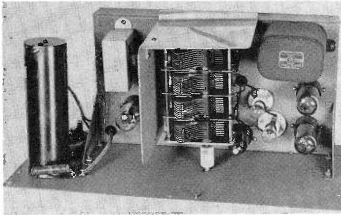
Interior view of capacitor-type R-C Oscillator.
