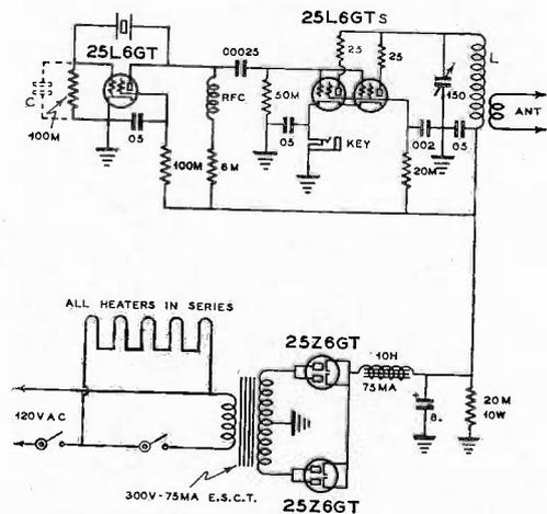
Simple circuit for a midget c.w. transmitter of improved design
