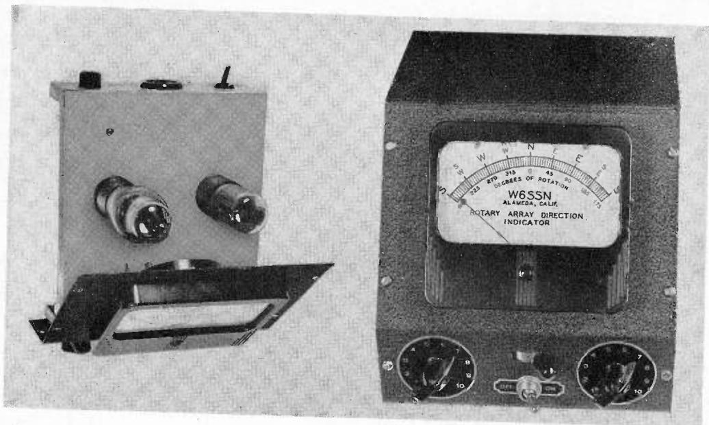
Interior and exterior views of W6SSN's rotary-beam indicating device.
