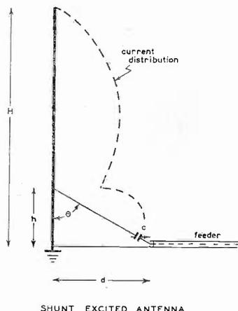
matched properly by varying the connection point on the inclined conductor, i.e., the distance  $h$ . The capacity  $C$  can then be varied until the transmitter load becomes normal, and then the standing waves are minimized or eliminated from the transmission line.
