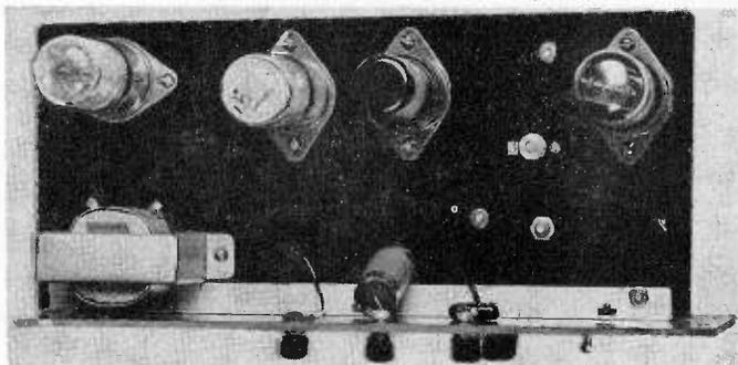
Looking down on the main inner panel of the Frequency Standard.
