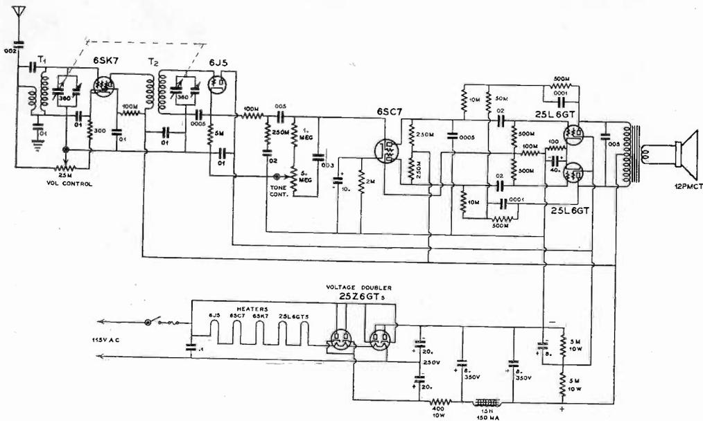
Schematic wiring diagram of t.r.f. tuner, audio channel and power supply for up-to-date speech and music reproduction. The electrical constants of the audio circuit are critical and should not be changed.
