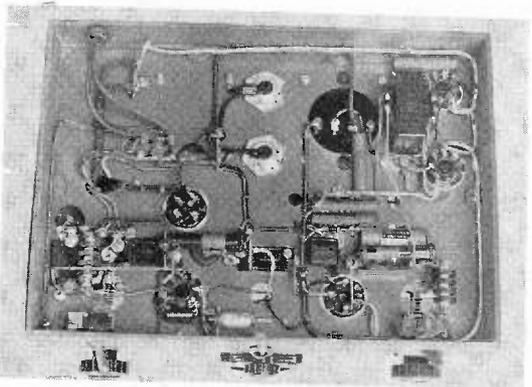
Bottom view of the 10-meter Transmitter. Note care exercised in layout and wiring.
