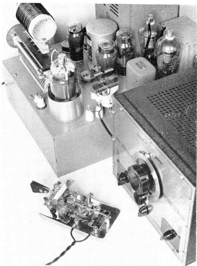
Rear view of the 813 beam tube transmitter and Meissner Signal Shifter. This medium-power compact ensemble can be quickly transported from place to place, and connected to the 110-volt a.c. mains anywhere—or to an auxiliary power plant—in order to establish emergency communication. The output of the transmitter is great enough to insure a powerful signal at the receiving point, a distinct advantage for reliable communication when and where it is needed.
