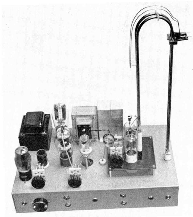
The complete 2 1/2-meter transmitter and hair-pin rod assembly.
