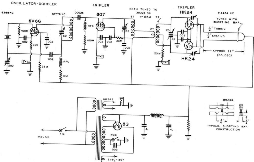
Circuit diagram of r-f portion of 2½-meter crystal-controlled transmitter.
