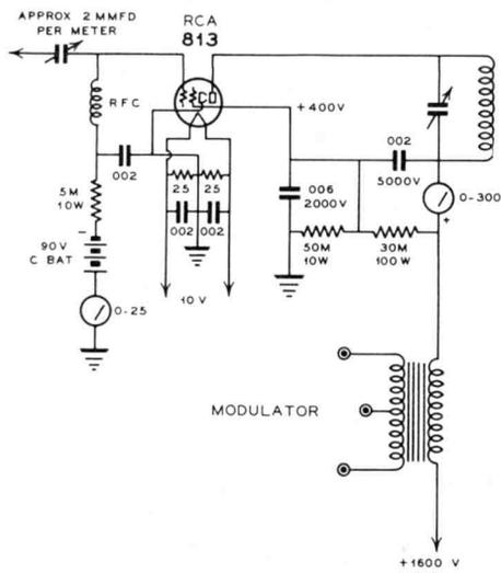
The final r-f amplifier can be biased for c.w. or 'phone operation in the manner shown above. This method is to be preferred over that shown in the tube bulletins.
