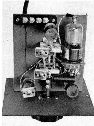
Looking into the 10-meter converter. Note mounting of tube and small components to facilitate short leads.
