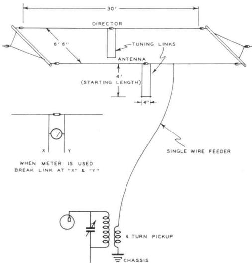
Constructional details of the wire-element, two-band, single-wire fed beam antenna.
