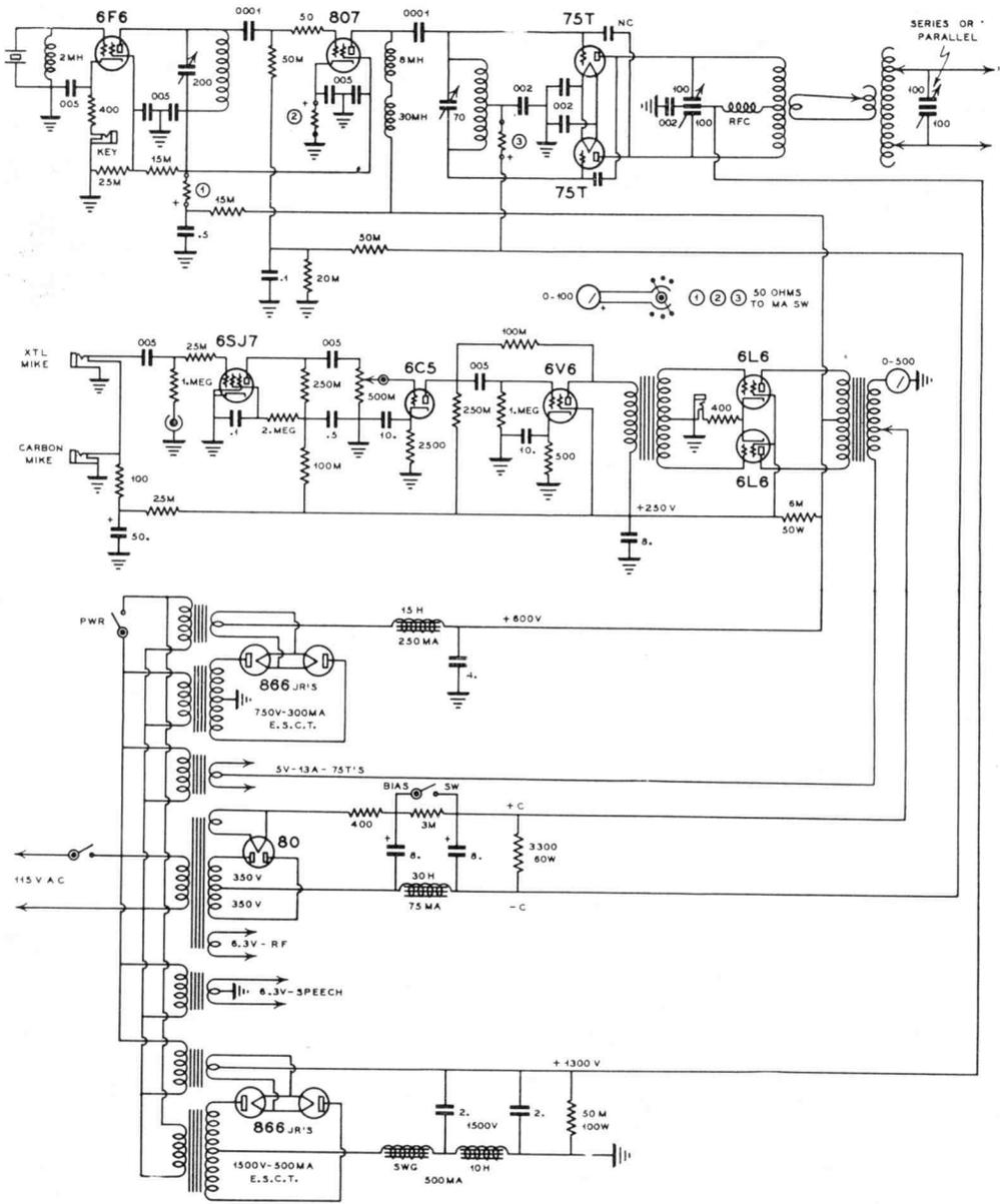
Schematic wiring diagram of 250-watt cathode-modulated 'phone and 500-watt c.w. transmitter.
