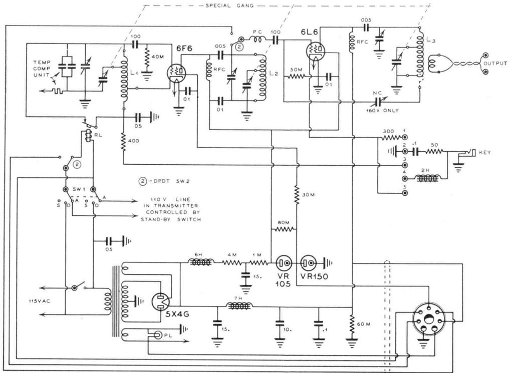
Fig. 1. 1941 Signal Shifter—Circuit Diagram
