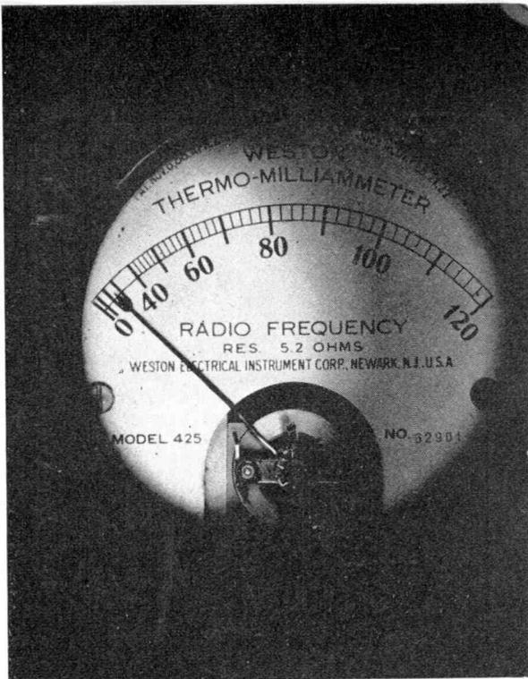
Figures don't lie. The r-f thermo-milliammeter indicates the low value of crystal r-f current in the new Wells Oscillator. Many crystal cuts were tried in this new circuit; all gave satisfactory performance—even the low-cost variety.
