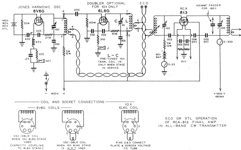
Complete schematic wiring diagram of the 813 beam-tube transmitter and supplementary sketches showing coil connections for ECO or crystal operation.
