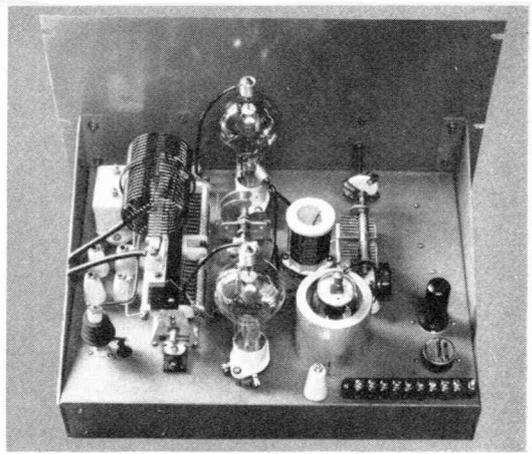
Only two chassis are required for the exciter, final r-f amplifier, speech channel and its power supply. The illustrations show the principal components for a compact medium-power cathode-modulated transmitter, described in the text.
