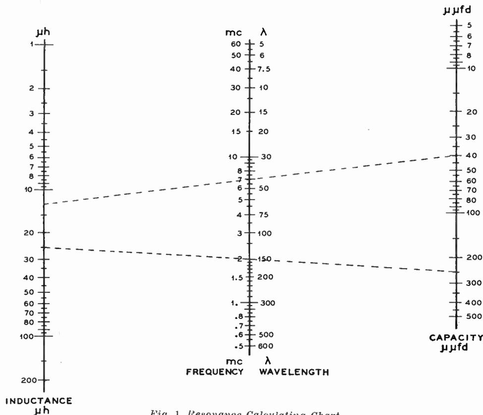
Fig. 1. Resonance Calculating Chart.
