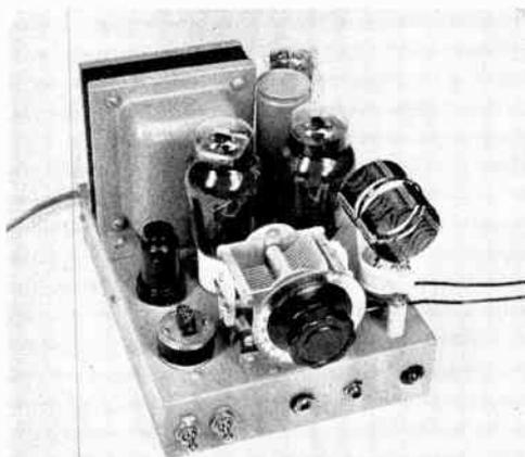
Complete C.W. Transmitter and Power Supply—ready to operate.
