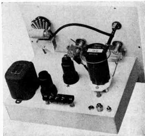
*Rear view of the little “bloofer,” showing details of tuned antenna circuit for greater selectivity and better signal strength. Connection to antenna coil,  $L_1$ , is by means of a pair of leads secured to the bakelite arm which rotates the coupling coil. This coil has one turn of wire, coupled loosely to coil  $L_2$ .*
