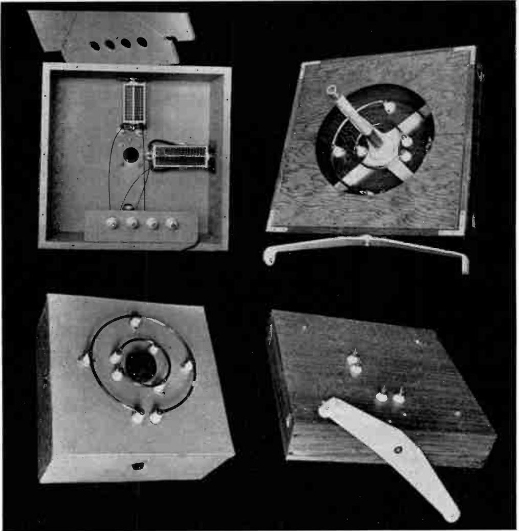
Rotary beam inductive coupling system for top-of-tower mounting. This device will be treated in a subsequent issue of the magazine. Several innovations in "compass boxes" will also be covered.
