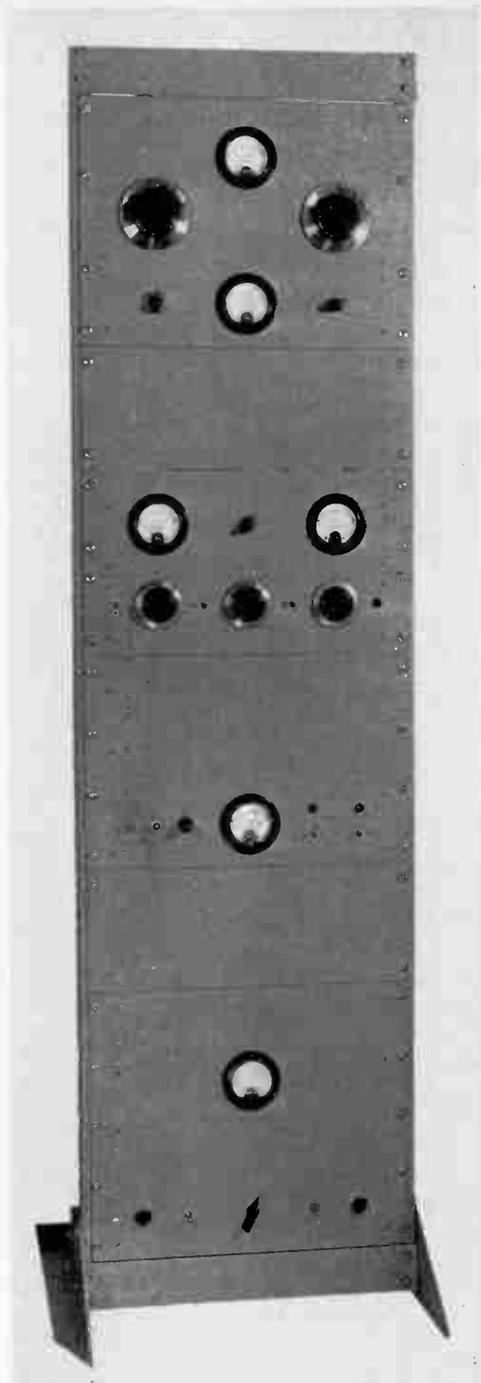
Semi-High Power, High Frequency 'Phone-C.W. Transmitter with HK-254 Gammatron Push-Pull Final Amplifier
