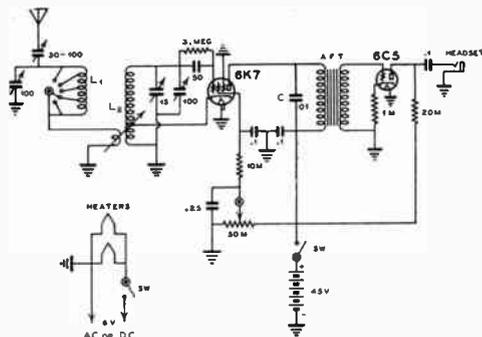
*Schematic wiring diagram of highly-selective battery-operated “bloofer.” Values of components should not be changed. The audio transformer is a conventional 3:1 unit.*
