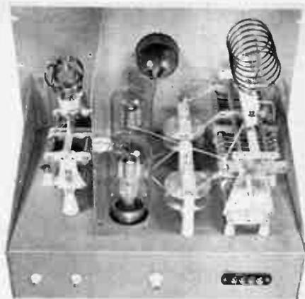
Two views of the final r-f amplifier deck, top and bottom of chassis. The grid circuit is shielded from the plate circuit by means of a large aluminum baffle.
