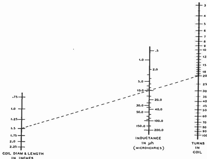
Fig. 2. Coil Calculating Chart.
