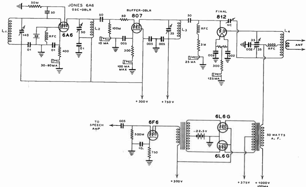
Fig. 1—Schematic wiring diagram, with circuit constants, for r-f portion of 100-watt transmitter—also a suitable low-cost modulator stage.
