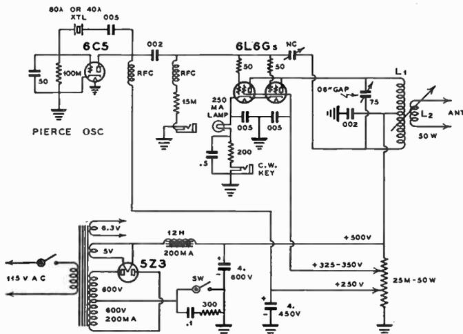
An inexpensive, compact stand-by c.w. set, complete with power supply, on a single chassis. More than 75 watts input. An ideal small transmitter for the 'phone men who wish to keep up with their code speed.
