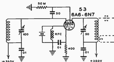
Fig. 2—Standard 6A6 oscillator-doubler circuit, the output of which is on the second harmonic of the crystal frequency.
