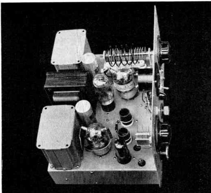
• Looking into the complete transmitter, the Millen tuning condensers are plainly shown. The power supply components are UTC, with specifications given in the schematic. The final amplifier shows a 10-meter coil in place.
