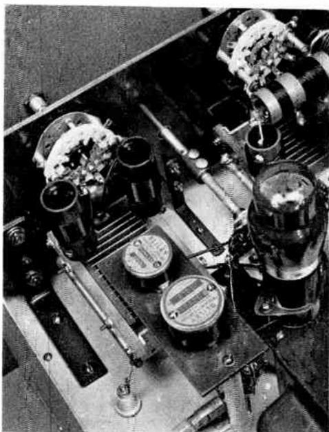
*Jones harmonic oscillator with tapped coils and rotary switch for multi-band operation. Two crystals enable the oscillator to deliver output from 160 to 20 meters. A small rotary switch selects either the 160- or 40-meter crystal. Both sides of the crystal are either in or out of service—rather than cutting-in or out the grid connection only.*
