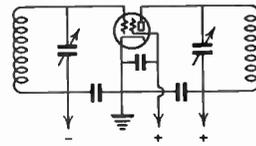
FRAMEWORK ACTING AS LINK COUPLING BETWEEN INPUT AND OUTPUT CIRCUITS.
