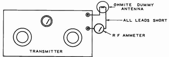
Fig. 3—Dummy Antenna Replacing Untuned Line
