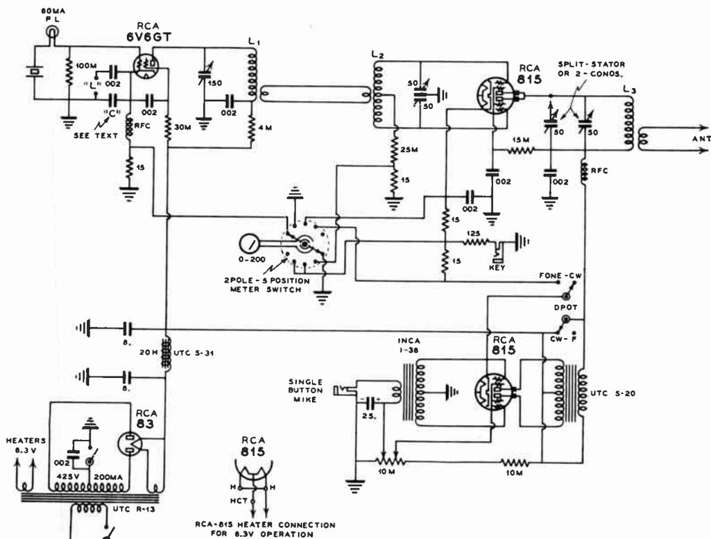
Complete Schematic Wiring Diagram of All-Band, 'Phone-C.W. Transmitter
