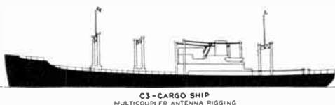
A single aerial is made to serve up to 21 individual sets through as many convenient radio outlets. Additional aerials are installed if more sets are to be accommodated. One tanker, the Esso "Nashville" for example, has three aerials serving 34 outlets.
