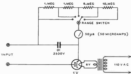
*Circuit diagram of the peak vacuum-tube voltmeter illustrated above.*
