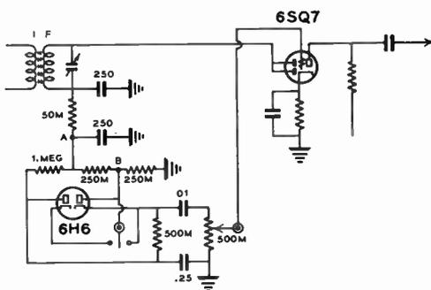
Fig. 1—New Series-Shunt Type Silencer
