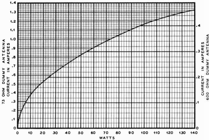
Fig. 10—Watts Versus Current for 73 Ohm and 600 Ohm Dummy Antennas
