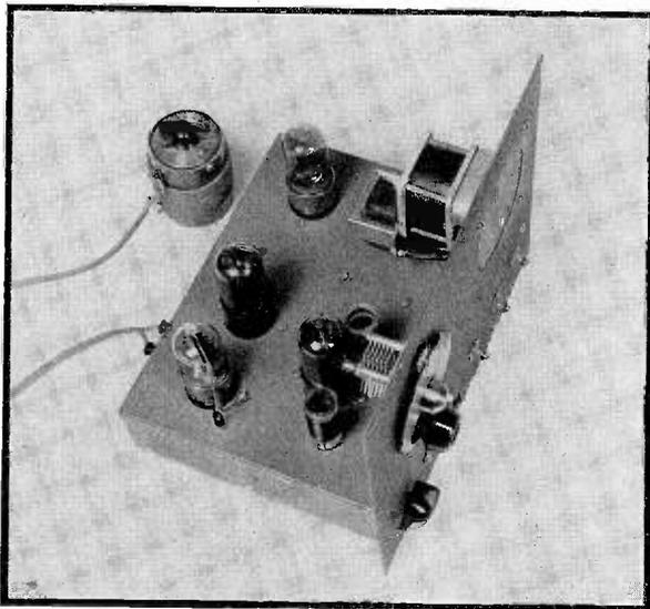
*Interior View, Showing Placement of R-F and Oscillator Coils, A-F Tube, and Loud-Speaker.*
