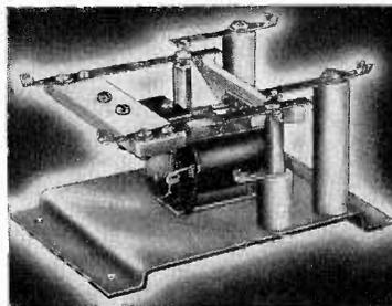
● A new relay designed for Amateur and Commercial use. Allows the use of the same antenna for transmission and reception. May also be used for making and breaking other R. F. circuits. Base and crossbar are of mycalex to keep losses at an absolute minimum. Has ceramic terminal posts. All contacts are widely spaced to prevent leakage and flashover. Actuating coil operates on 110 volts A.C. Relay measures 3" x 3" x 2" high over-all.
