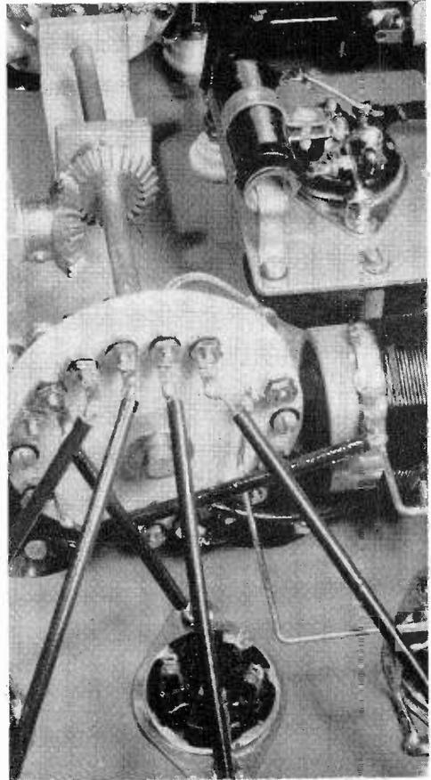
Typical example of engineering design for a band-switching unit in a commercial transmitter. From a photograph of Tecrad's marine application.
