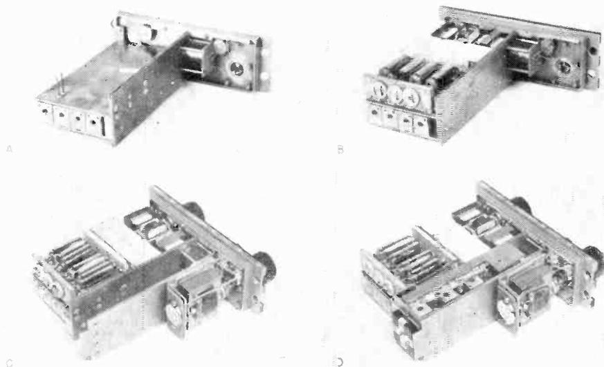
Subassemblies used in the new receiver. A shows tuning assembly and RF inductors in place. At B, RF amplifier and power-filter assemblies have been added. At C, output transformer, potentiometer, and other hardware are in place. At D, IF amplifier, input-output connector are installed and the set is ready to be sealed in its case. Audio output tube assembly is plugged on the outside of case for easy replacement.
