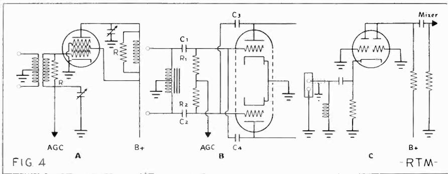
RF amplifier circuits commonly used in television tuners. Respectively, A, B and C are the conventional grid input circuit; the amplifier used in the RCA 630TS circuits; and the grounded-grid circuit. Grid acts as shield between input and output in circuit C.
