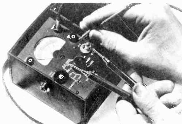
Miniature multimeter manufactured by International Instruments. The meter, although small in size, is large in utility; it has three DC ranges and three AC ranges at 10,000 ohms per volt, plus four resistance ranges.
