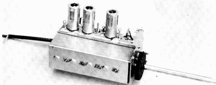
The "Teletuner," a complete front end built by Mallory around its four-gang "Inductuner" (see cut at bottom of page).
