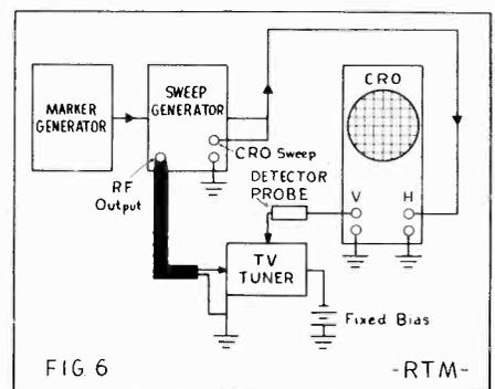
Connections between oscilloscope, sweep, and marker generators for alignment of TV front end.
