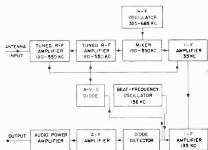
Block diagram of the subminiature set. Conventional superhet circuit is used.
