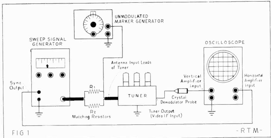
Setup for observing the response of the TV tuner to the input signal. Tests are easier if tuner is removed from the main receiver chassis.
