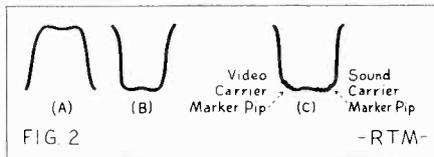
Tuner response curves may be upright or inverted on the scope face.
