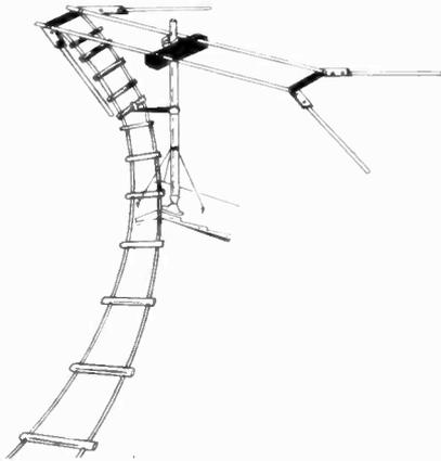
twin leadin. Released figures show 0.5 Db loss per 100 feet at 200 Mc, making possible longer line installations in remote and fringe areas.
