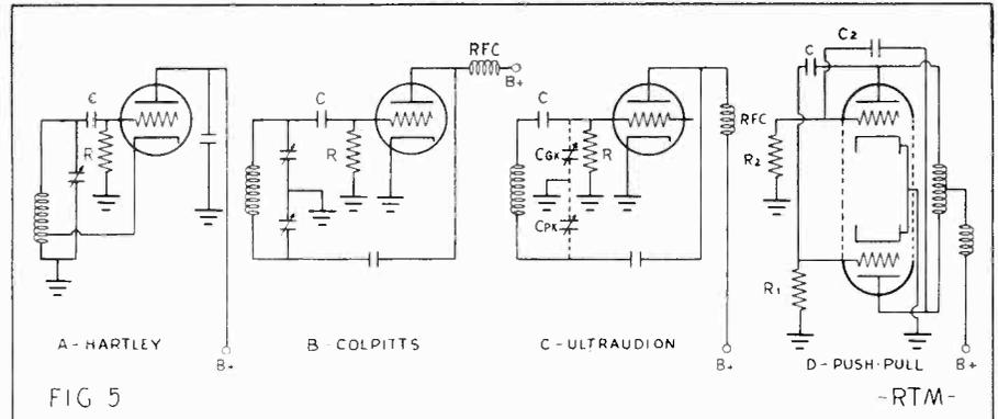
Representative circuit arrangements used for the local oscillators of television receivers. Note similarities of first three circuits. Most commonly used is the ultraudion shown at C.
