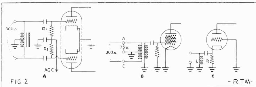
Television input circuits. At A, a balanced 300-ohm input is shown, with a center-tapped choke. Circuit B shows an input with choice of either 300- or 75-ohm input, balanced one way, and unbalanced the other. At C, the 75-ohm input is into a grounded-grid RF amplifier. Input impedance depends largely on the value of resistor R.
