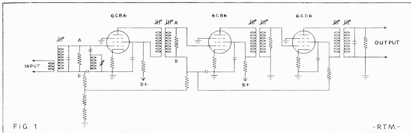
Test points on the grid resistors of video IF stages. Service procedure with only VTVM and other basic field equipment (see text) will usually
