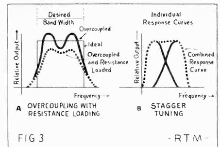
Methods of broadening the response curve of a TV stage.
