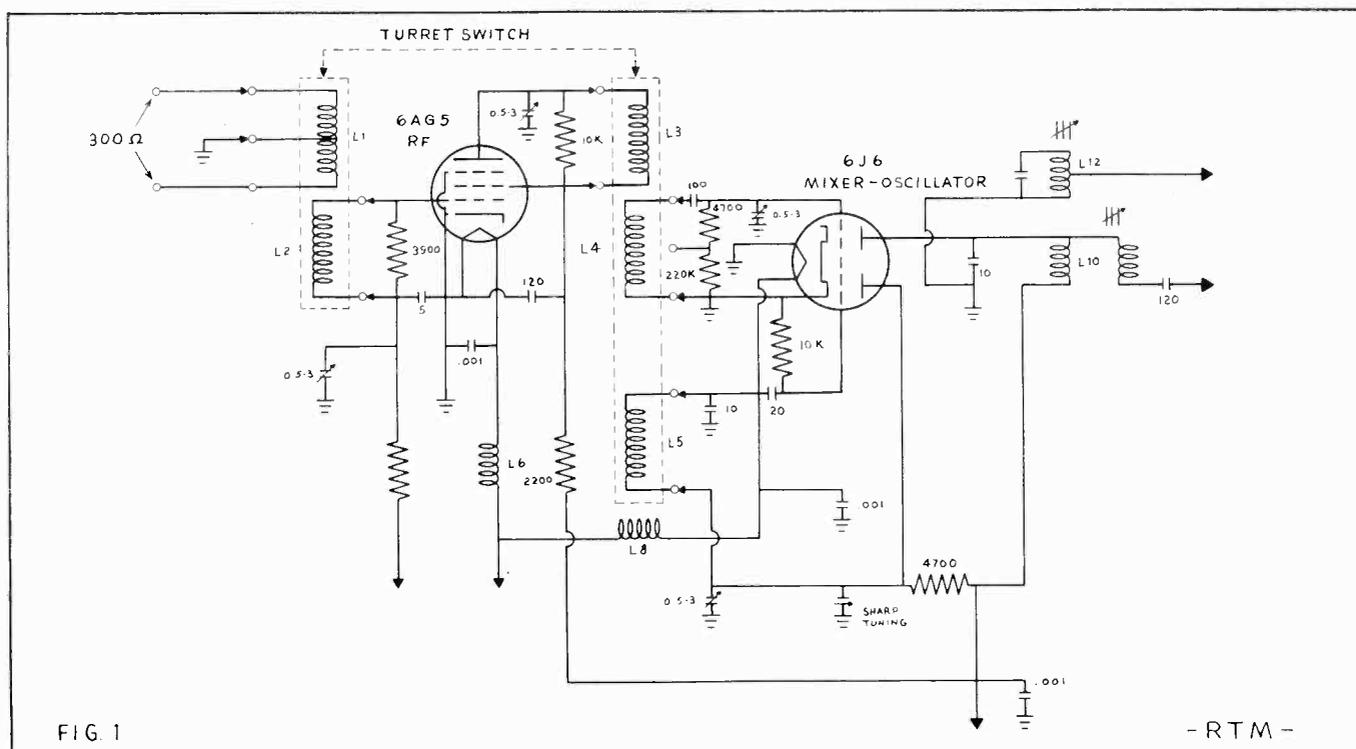
Circuit of the widely-used Standard Tuner. In this turret-type unit, different coils are switched into the circuit for each channel. Note interchange
