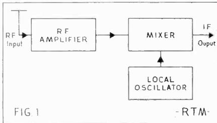
Block diagram of a typical TV tuner.
