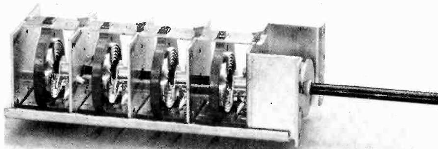
The four-gang "Inductuner." Note mechanical simplicity of this unit, which is a basic tuner for front-ends built by several companies in addition to Mallory. Shorting fingers and spiral inductances can be seen in this picture.
