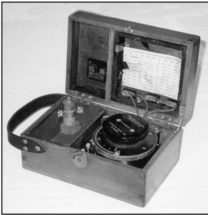
Figure 2. A Marconi Wireless Telegraph Co. Wavemeter in its case after restoration by the author.
