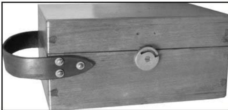
Figure 3. This view of the Wavemeter, with its cover closed, shows its dovetail construction and excellent restoration.
