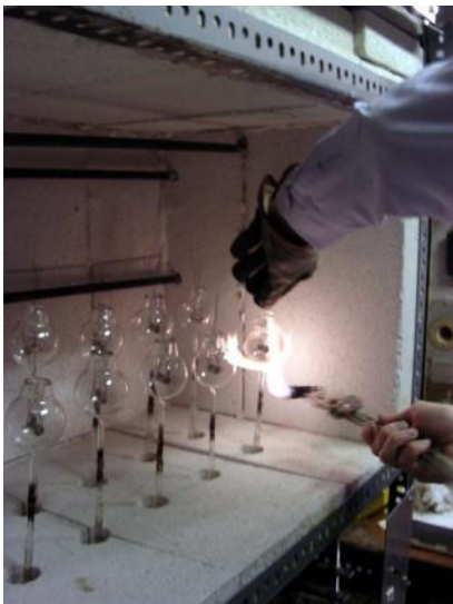
34 Melting off the tubes
