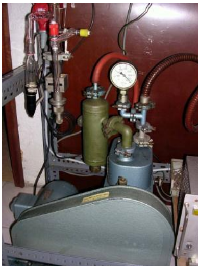
23 Two step rotating pump
