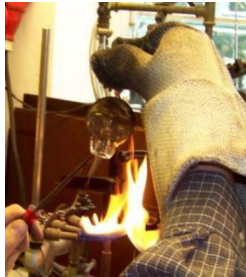
20 Removing the bulb with the melted-in system from the tool
