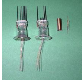
14 Press ready for mounting the system
