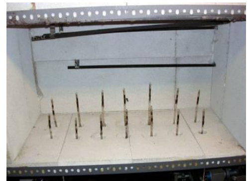
28 View into the pumping oven
