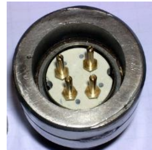
38 Base before pressing in the tool
