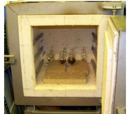
21 tubes in the cooling oven
