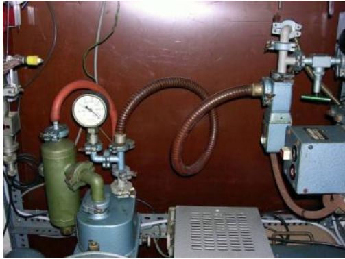
26 Connection of rotating pump and diffusion pump
