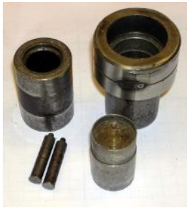
37 Tool for pressing the base
