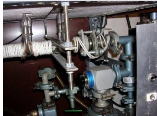
25 Vacuum rack connected to the diffusion pump
