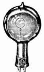
It is of the gas-filled, potassium magnesium type, employing a special set-back anode to increase its output. Individually tested during and after construction for sensitivity and uniform frequency response. Its fairly low ionization point reduces battery noises to a minimum. The bases are of bakelite UX 4 prong type. Information as to characteristics furnished on request.
