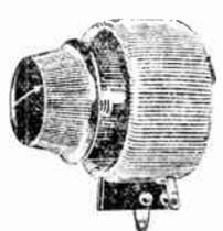
The wire-wound resistance is built of materials that insure safe operation at high temperature. The wire is wound on a steel core, 1" wide, which is insulated with asbestos. The diameter is 2" which allows mounting the unit in a comparatively small space. This construction provides a resistance unit that will safely carry any current load at a power dissipation of 50 watts through the entire resistance.
