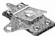
A sturdy, accurate neutralizing, balancing or trimming condenser—very small and compact—for use in balancing multiple-tuned circuits or equalizing separate condensers "ganged" for single control. Adjustment of center screw provides even, gradual capacity change over a wide range. Fits into recesses in multiple condenser frames or may be attached directly to binding post of socket or condenser. Best mica dielectric, heavy phosphor bronze spring plate. Highest quality insulating material base.
