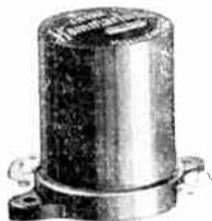
The radio frequency chokes which have been for years recognized as standard throughout the radio industry. Manufactured by special process of winding and impregnating. No resonant period within broadcast band. Low distributed capacity makes them unusually effective for short-wave work. Ideally suited for use in detector plate circuits, B plus and grid return leads of radio frequency tubes and any other place where R. F. filtering is required. Current
