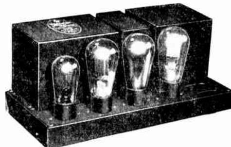
Model BD-27-45 is designed for use with a D. C. Dynamic Speaker, without input transformer, having a field coil D. C. resistance of 1800-2000 ohms. To use an A. C. Dynamic Speaker the CR-35-B choke-resistance unit should be connected across the field terminals of the amplifier.
