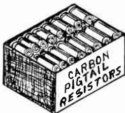
The Resco Carbon Resistor Kit is composed of 29 carbon pigtail resistors, one each of the popular sizes. A handy kit that should be had by all radio servicemen and dealers.
