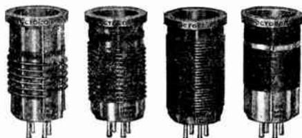
For the amateur or short wave fan Octo-Coils are the most rugged coils built. Very efficient in operation and fit standard four prong tube sockets. Moulded of genuine bakelite in four distinctive colors: Green, brown, blue and red. Designed for use with .00014 Mfd. tuning condenser. Wave length range for coils, 15 to 200 meters.
