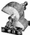
Size 1 1/2" x 1 1/4" x 2". Standard SE-100, capacity 100 mmf., 10 rotor and 10 stator plates. Rotor and stator plates readily removable to alter capacity range to meet special circuit requirements.
