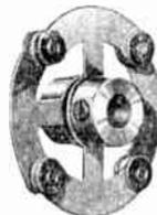
An ideal coupling for radio condensers. Permits operation of any number of variable units in tandem without requiring exact shaft alignment. Saves time, money and worry. Sides of coupling are insulated from each other, allowing instruments in gang to be operated as independent electrical units. Tough baked canvas, with brass bushings and hardened set screws.
