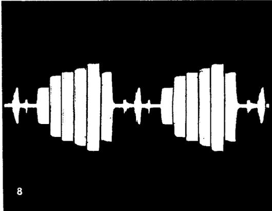
luminance amplifier. If the waveform is not symmetrical to the axis, an incorrect operating point of the chroma amplifier may be the reason, e. g. leaky coupling capacitor between luminance and chroma amplifier or too small a control voltage at the chroma amplifier. Fig. 7 shows an unsymmetrical waveform of the chroma signal, caused by the wrong operating point of the first band-pass amplifier. (Control voltage too small.)
