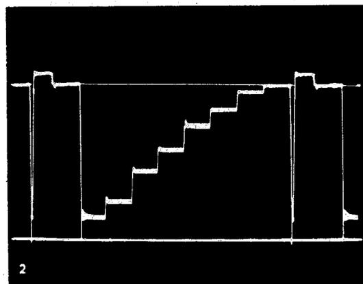
luminance signal and fig. 2 a distorted gradation trace caused by insufficient AGC voltage in the IF-amplifier. In many cases it would be possible to notice this fault on the picture without a CRO. It is recommended that the field hold be adjusted so that field blanking is visible on the screen. The degree of black level between field sync pulses and field blanking will give a very good indication of pulse clipping. However one can not identify the stage where the fault is present.
