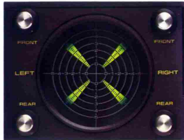
4 channel level indicator on QX-949 A.
