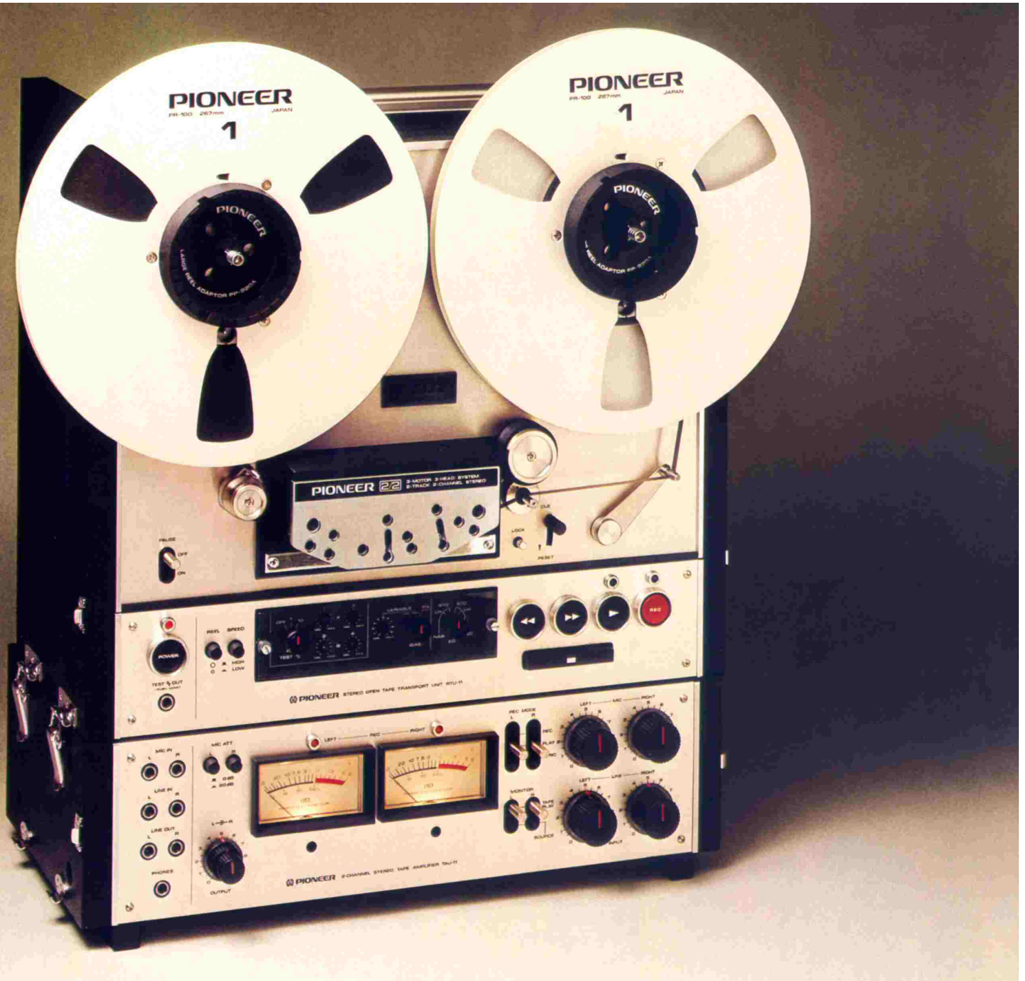
RT-2022: Professional open reel tape system. 2 tracks. 2 channels, 3 motors. Capstan drive. 38 cm/sec. and 19 cm/sec. Wow and flutter: no more than 0.04 % (JIS). Signal to noise ratio: more than 57 dB. Frequency reponse: 30 Hz to 28 kHz ( \pm 3 dB at 38 cm/sec.). Separate read unit. Separate record and playback amplifier.
