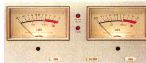
Wide range scale level meters and peak level indicator on CT-F 8080.
