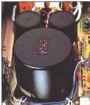
Huge toroidal core transformer of SX-1080.
