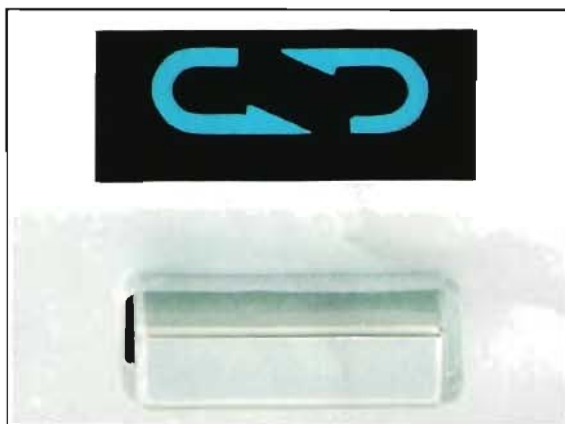
Display window of CT-F 750 indicating it is set in auto-reverse and repeat mode for endless play.
