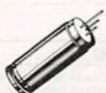
A low power collimator pen containing a MOVPE grown gain GaAlAs laser. This collimator pen delivers a maximum CW output power of 2.5 mW at 820 nm. The operating voltage of 2.2-2.5v @ 90-150mA is designed for lower power applications such as data retrieval, telemetry, alignment, etc.
