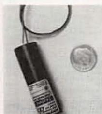
The LDM 135 integrated assembly consisting of a laser diode, collimating optics and drive electronics within a single compact housing. Produces a bright red dot at 660-685 nm. It is supplied complete with leads for connection to a DC power supply from 3 to 5.25 V.
