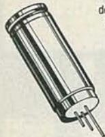
A low power collimator pen containing a MOVPE grown gain guided GaAlAs laser. This collimator pen delivers a maximum CW output power of 2.5 mW at 25°.
