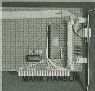
A computer by itself can't do much; it needs some way of communicating with the outside world. It needs to be able to sense external conditions (a switch closure, for example), and it needs to be able to control circuitry (a relay, for example). The principles of interfacing those types of devices are not difficult; we'll show how easy it is by building an experimenter's card for the IBM PC expansion bus.
