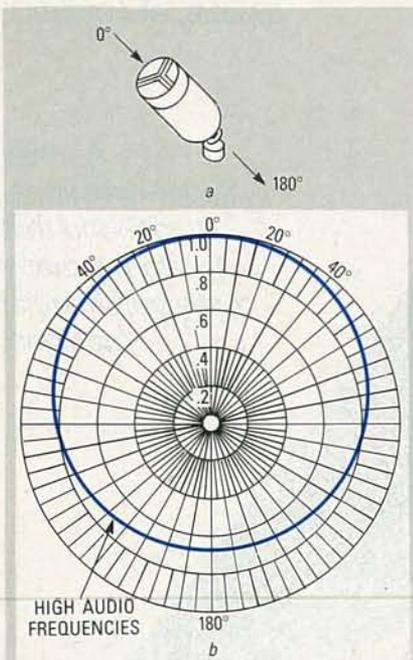
FIG. 1—AN OMNIDIRECTIONAL microphone, shown in (a), has uniform directional sensitivity to sound pressure  $P(\theta)$ ; the main axis is out the indicated. In (b) is shown a polar plot of directional sensitivity; the response is identical in any plane through the main axis.
