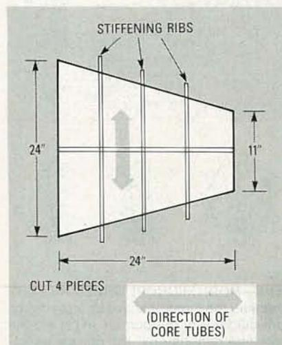
**FIG. 14—HORN EXTENSION CUTOUT; the ribs stiffen the cardboard. The extension slips over the horn, extending its length and expanding its mouth, and two 1/4-20 screws with washers hold both together. The mouth is now 2 × 2 ft, one wavelength across at  $f = 557.742$  Hz, matching wavelengths down to lower audio frequencies, improving directivity, raising the pressure level by 3 dB, and providing better low-frequency pick-up, since impedance matching is improved.**
