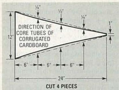
**FIG. 11—HERE'S THE CUTOUT FOR ONE side of the basic horn; note the direction of the corrugated ribs. The edges have slight curvature so the sides have added strength, and don't resonate easily. The edges were taped, and paper glue was used on the inner and outer corners. The small end was cut to a 1-inch diameter, and the microphone slides in and is held by the four sides. A metal washer slipped into the throat face acts as a stop, yet lets the sound reach the diaphragm.**
