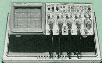
WHAT DO YOU GET WHEN YOU CROSS A 20-MHz, 4-channel oscilloscope with four digitizers and an RS-232 interface? You get the 2214 Digital/Analog oscilloscope from Tektronix (P.O. Box 500, Beaverton, OR 97077).
