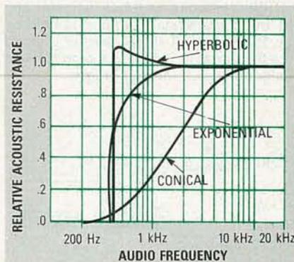
FIG. 9—RELATIVE ACOUSTIC resistance for several horn microphones of size and bandwidth similar to Fig. 6. Each works just as well as a loudspeaker by reciprocity, with the exponential, hyperbolic, and conical the most common.
