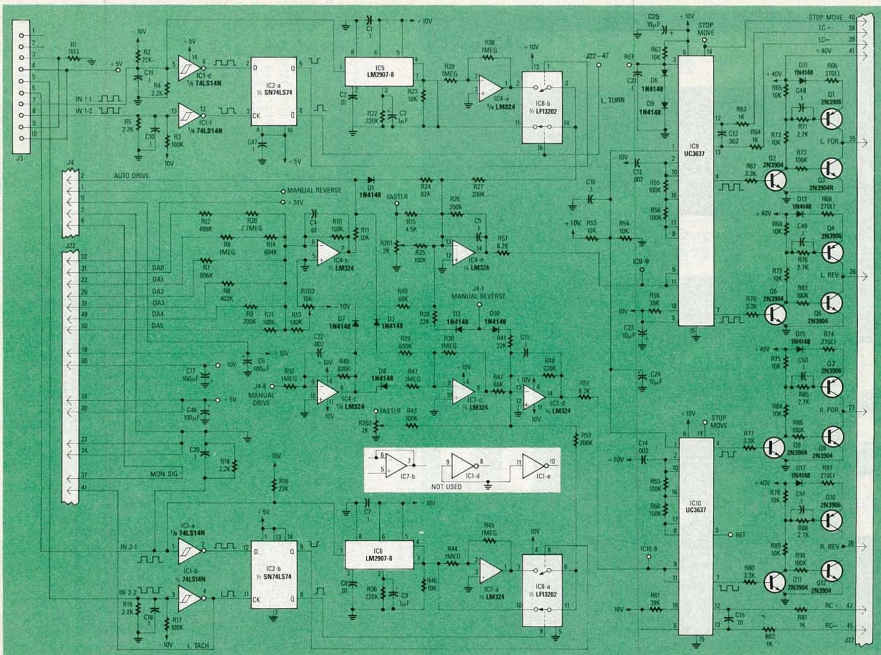
FIG. 3—PARTIAL SCHEMATIC DIAGRAM of the motor-controller board.
