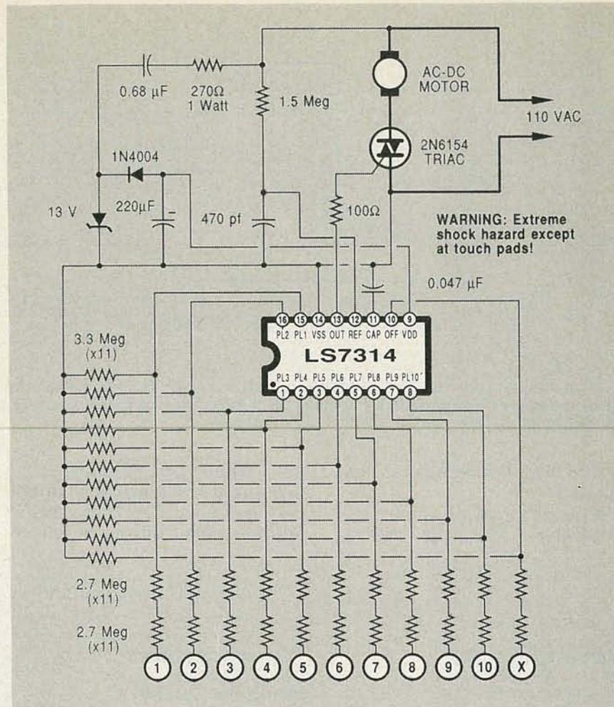
**FIG. 4—A 10-SPEED TOUCH-CONTROL BLENDER circuit that uses the low-cost LS7314 chip by LSI Systems. The eleventh touch pad is for power off.**
