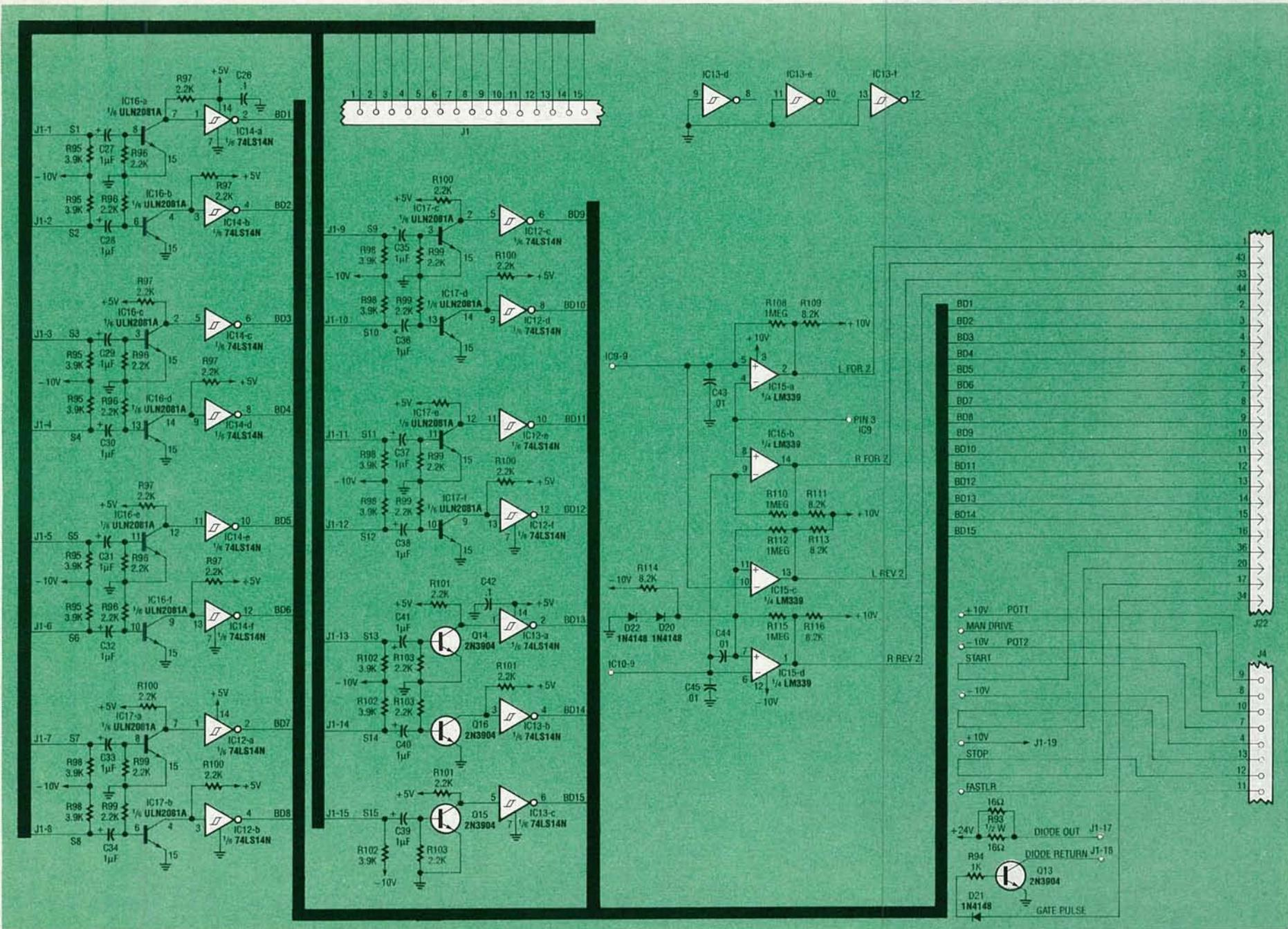
FIG. 4—THE GRASS-SENSOR AMPLIFIERS are located on the motor controller board.
