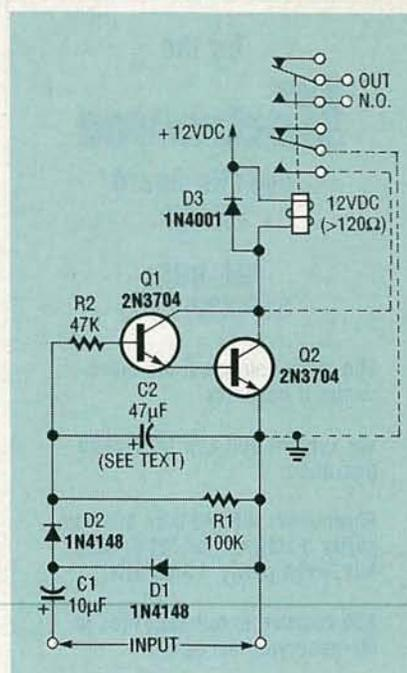
FIG. 13.—SIMPLE RELAY-OUTPUT sound- or vibration-sensor system.
