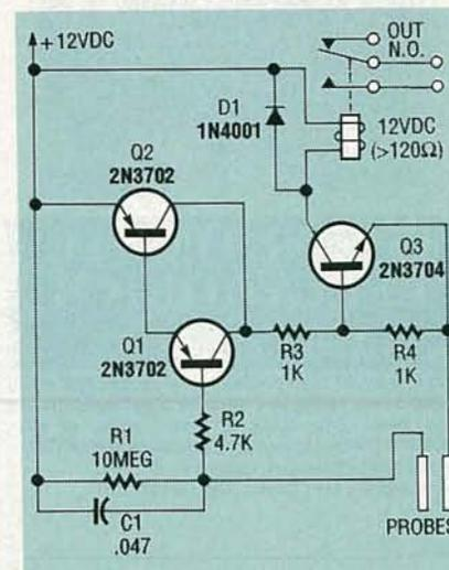
FIG. 15.—SENSITIVE FLOOD-ALARM system with relay output.
