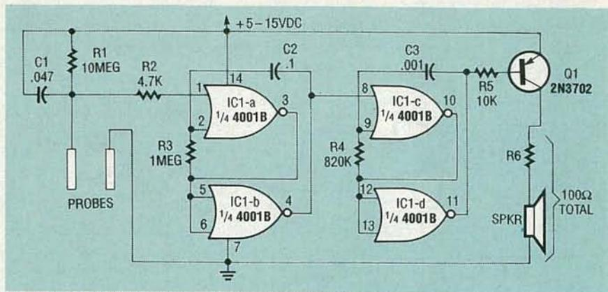
FIG. 16.—SENSITIVE PULSED-TONE flood-alarm system.
