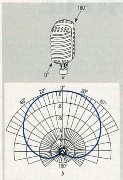
FIG. 2—A CARDIOID MICROPHONE, shown in (a), has greater sensitivity from the front than the rear. The  $0^\circ$  and  $180^\circ$  directions are along its main axis, pointing through the main face. The sound pressure sensitivity  $P(\theta)$  shown in (b) was taken through a plane normal to the main axis.
