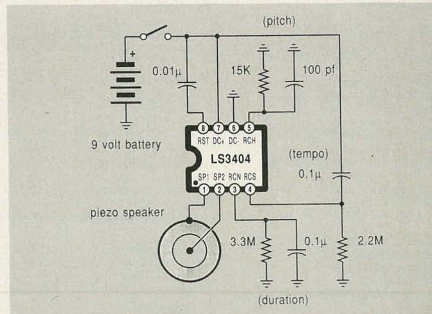
**FIG. 5—A HIGH-QUALITY MELODY circuit. The slow decay waveforms produced will create chime-like notes. Pitch, tempo, and duration are all adjustable.**
