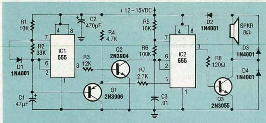
FIG. 8.—"RED-ALERT" SIREN simulating "Star Trek" alarm signal.
