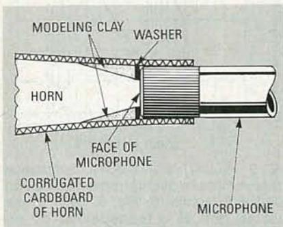
**FIG. 12—WHEN MOUNTING THE microphone in the horn, the washer aperture should be at least 75% of the diaphragm diameter. The modeling clay smoothed the transition from the square horn to the washer opening, so that the sound wasn't restricted from reaching the diaphragm.**
