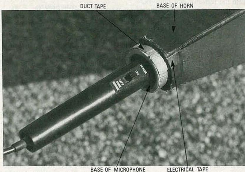
**FIG. 13—A CLOSE-UP VIEW OF THE EXTERIOR of the neck. The cardboard is tapered, producing an opening of proper size for the microphone, and the microphone is inserted. Note the silvery ring at the base of the horn, just behind the base of the horn. The bottom of the microphone protrudes from the base of the horn, and was sealed mechanically and acoustically with duct tape, while the base of the horn was stiffened with electrical tape.**
