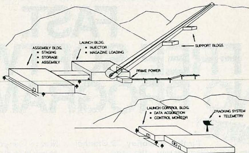
**A FUTURE FULL-SCALE EARTH-TO-ORBIT** electromagnetic launch system might look like this. The flyway, consisting of hundreds of stages, is built up the side of a hill to present a 30-degree launch angle.
