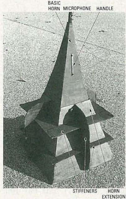
FIG. 15—HERE'S THE COMPLETED HORN MICROPHONE. At the top is the receptor microphone, then comes the basic horn, and lastly, the horn extension is shown with its support ribs.
