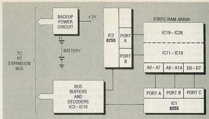
FIG. 1. THE STATIC RAM DISK consists of three major subsystems: an array of as many as sixteen 32K CMOS static RAM's, a bus-interface circuit, and a battery-backup circuit.
