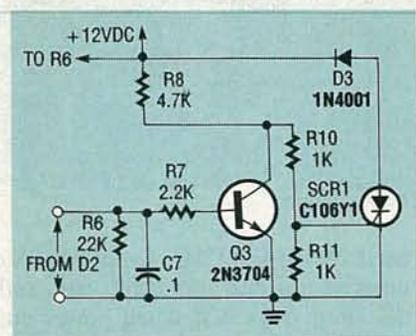
FIG. 11.—ALTERNATE DIRECT OUTPUT stage for the circuit shown in Fig. 13.
