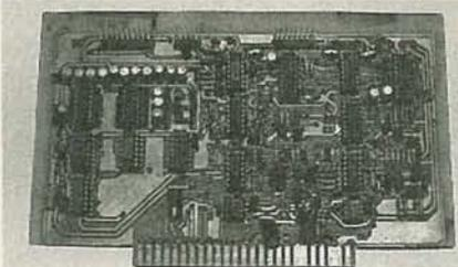
**FIG. 5—THE MOTOR-CONTROLLER board fits in one of the motherboard's slots.**
