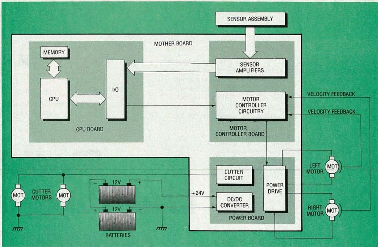
FIG. 1—BLOCK DIAGRAM of the electronic control system.
