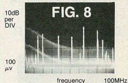
The same signal is then applied to the Spectrum Probe<sup>®</sup>. (20 dB atten. added to keep RF components within the logarithmic range.) Two major problems are visible in fig. 8. Why are very high spectral line levels present which are approximately 15 MHz. apart? The other problem, which can't be shown easily in the photo, is the alternating amplitude of the spectral line components — which indicates that significant low frequency components are present in the signal.
