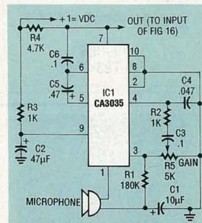
FIG. 14.—SPEECH-FREQUENCY AMPLIFIER used in conjunction with the circuit of Fig. 16 to make a sound-activated sensor system.
