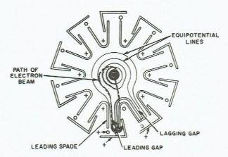
NOTE: STATIC - ONE SPADE AT CATHODE POTENTIAL
