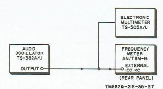
Figure 39. Test setup for external 100-kc input test.
