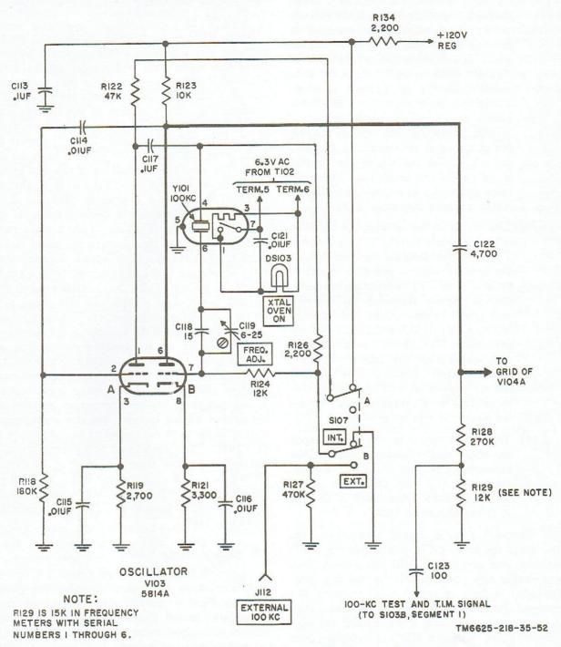
Figure 10. Crystal oscillator stage V103, schematic diagram.
