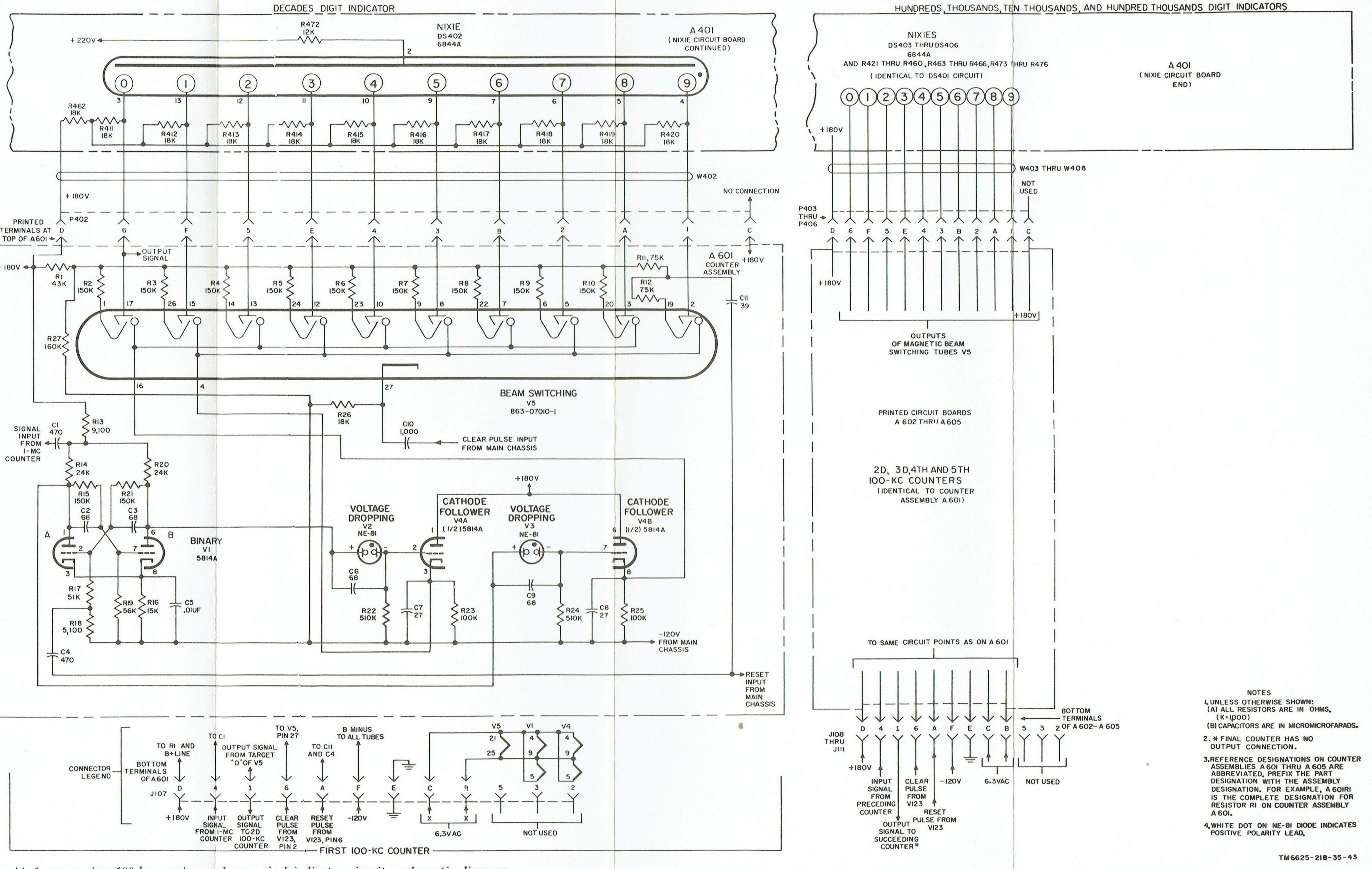
Figure 44. 1-mc counter, 100-kc counter, and numerical indicator circuits, schematic diagram.
