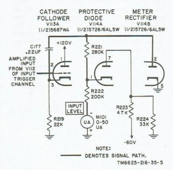
Figure 4. Meter circuit, schematic diagram.
