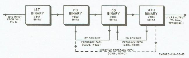
Figure 15. Clock counter A 301, simplified block diagram.
