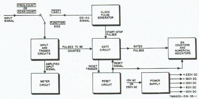
Figure 1. Simplified signal path, block diagram.
