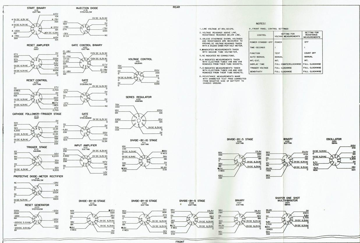
Figure 23. Tube socket voltage and resistance diagram, main chassis, bottom view.
