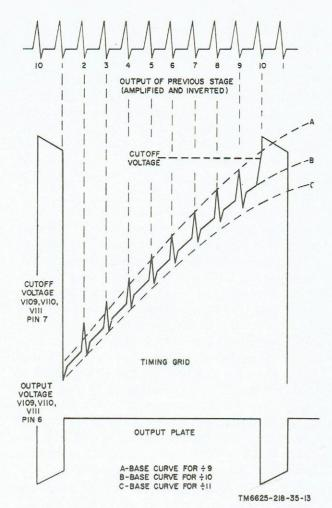
Figure 13. Divide-by-10 stages V109, V110, and V111 waveforms.
