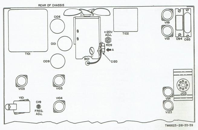
Figure 27. Top of main chassis, location of adjustment controls.
