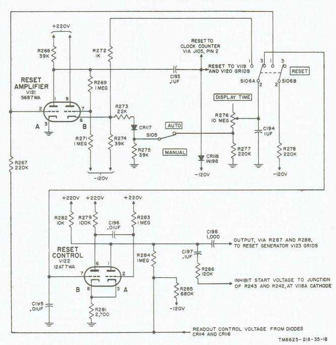
Figure 20. Reset amplifier and control circuit, schematic diagram.
