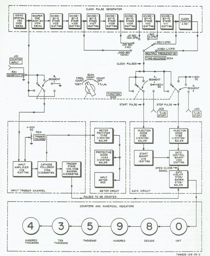
Figure 2. Detailed signal path for frequency counting, block diagram.
