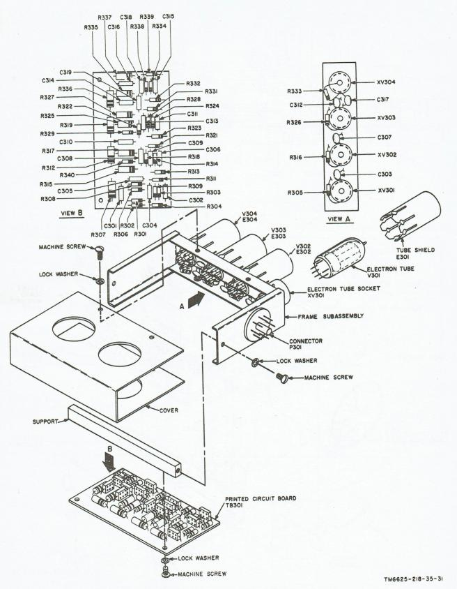
Figure 31. Clock counter assembly, parts location diagram.
