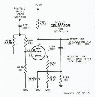
Figure 21. Reset generator V123, schematic diagram.
