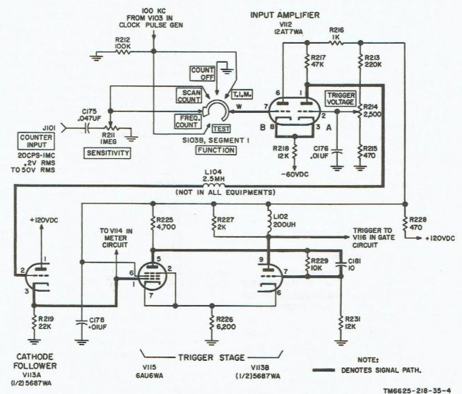
Figure 3. Input trigger channel, simplified schematic diagram.
