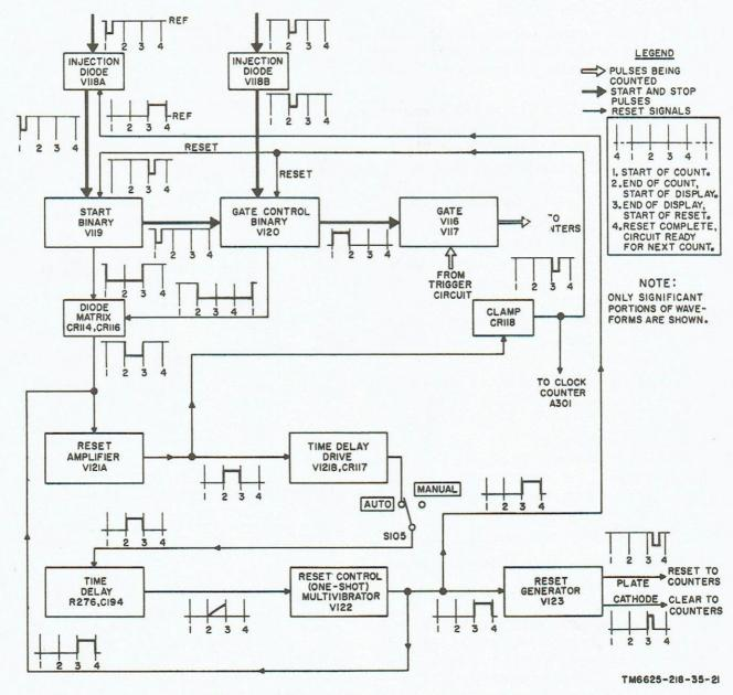
Figure 18. Reset circuit, functional block diagram.
