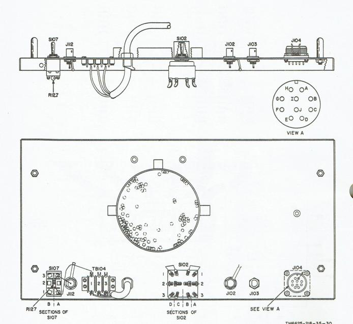
Figure 30. Interior of rear panel, parts location diagram.
