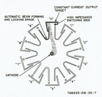
Figure 6. Beam switching tube array.
