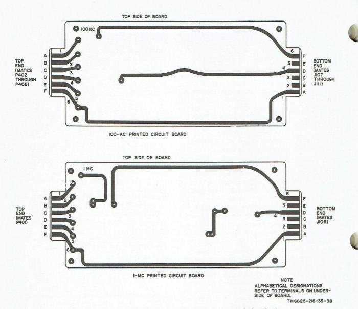
Figure 34. Counter assembly printed circuit boards, terminal identification.
