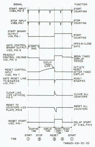
Figure 19. Reset control circuit, idealized waveforms.
