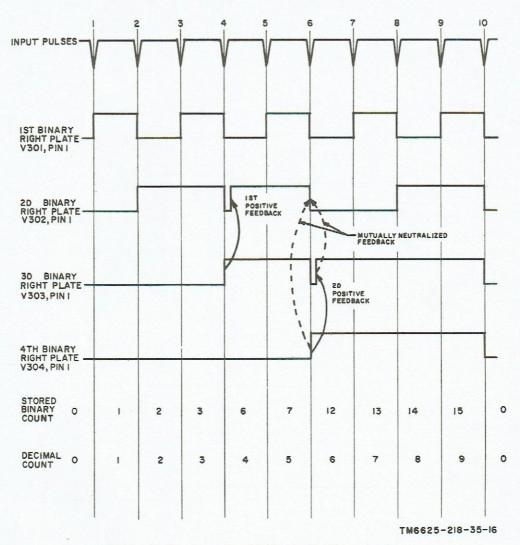
Figure 16. Clock counter A 301, idealized waveforms.
