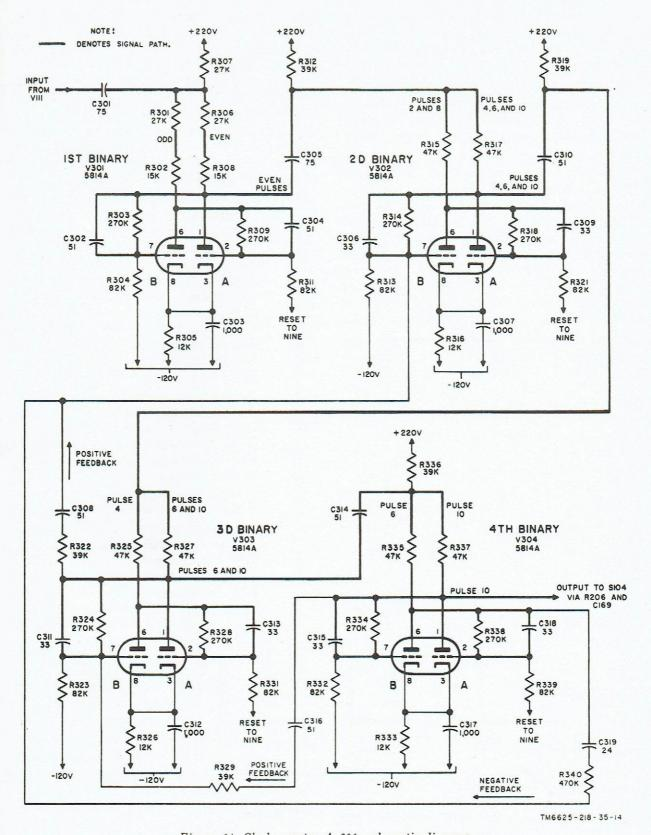
Figure 14. Clock counter A 301, schematic diagram.
