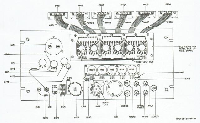
Figure 29. Rear of front panel, parts location diagram.
