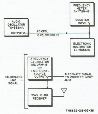
Figure 37. Test setup for frequency range, sensitivity, and accuracy tests.
