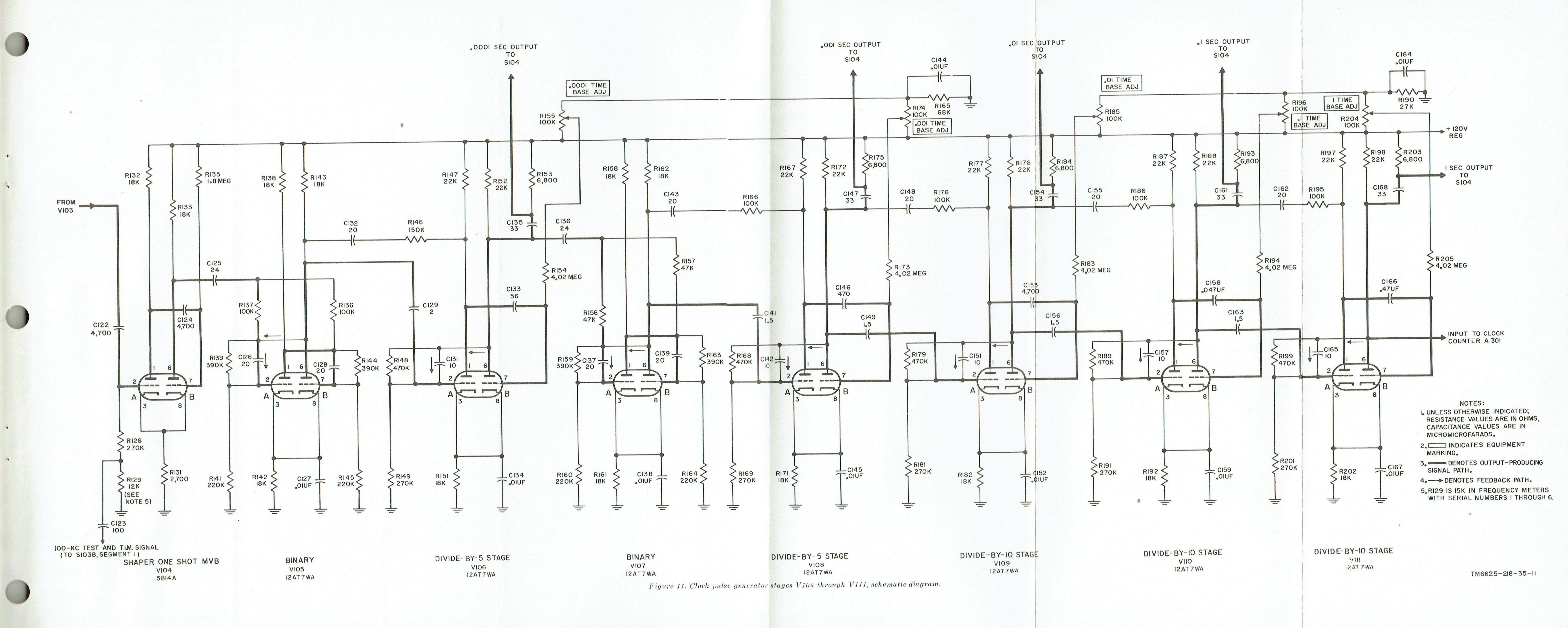
made less positive, less resistance is inserted in the discharge line, the capacitor will discharge faster, and division by the fourth trigger pulse may result. Resistor R165 is used as part of a voltage divider in the grid circuits of V106B and V108B and is also a factor in capacitor C133 and C146 discharge. Capacitor C144 also bypasses voltage variations to ground.
