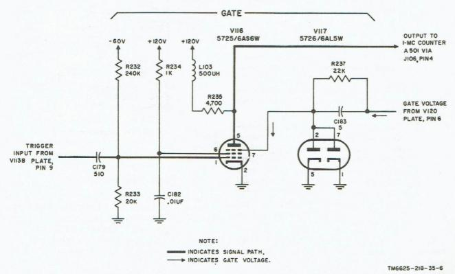
Figure 5. Gate circuit, schematic diagram.
