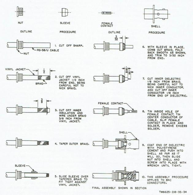
Figure 36. Assembly of rf cable and connectors.
