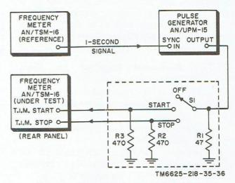
Figure 38. Test setup for time interval test.
