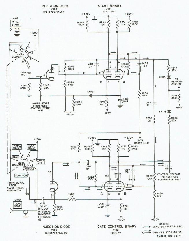
Figure 17. Gate control circuit, schematic diagram,
