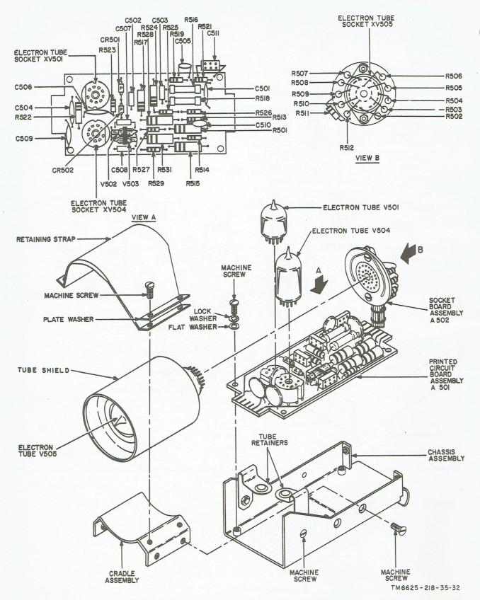
Figure 32. 1-mc counter assembly, parts location diagram.
