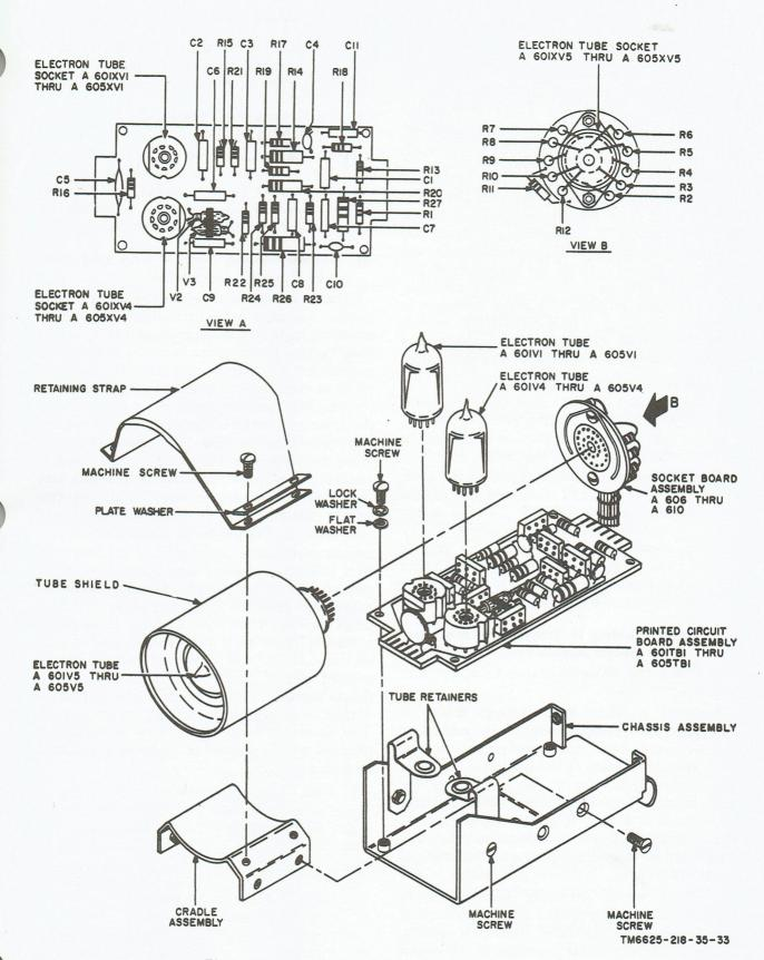
Figure 33. 100-kc counter assembly, parts location diagram.
