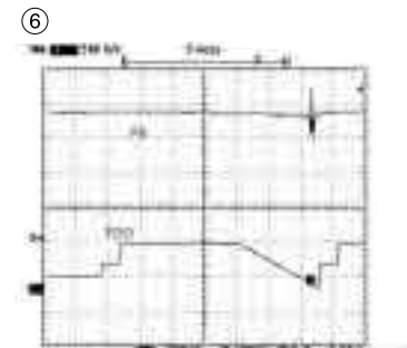
IC2A1 Pin42, Focus Error(in Focus Search) IC201 Pin 83, Focus Drive(FDO)
