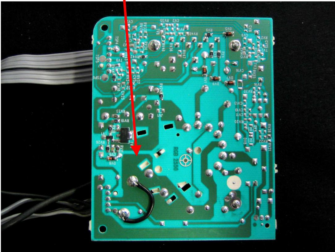
The indicated grounding path improvement is applied to production chassis (2550 and 8500) from June 2004 via a component side wire jumper.
