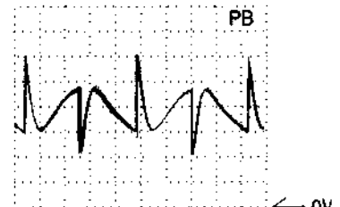
A: DC, 1 V/Div, 500us/Div Connector L9, 4
