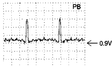
A: AC, 200mV/Div, 10ms/Div Connector L9, 3
