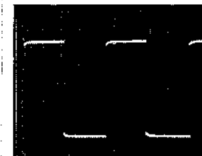
⑧ IC21 Pin 10 PB SP 1V/Div 50μSec/Div
