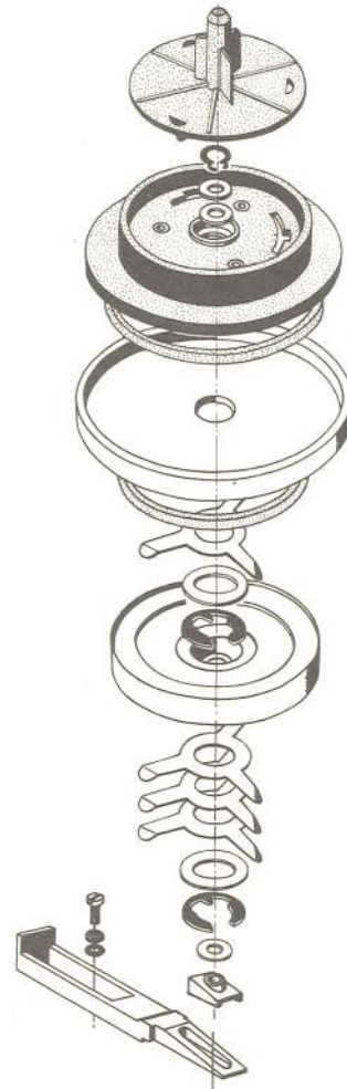
Fig. 3 Exploded drawing of the take-up plate (right)
