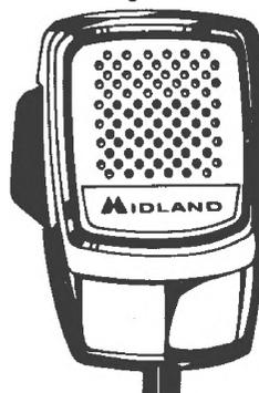
**Step 8:** To transmit, press the push-to-talk bar on the microphone. To receive, release the bar.
