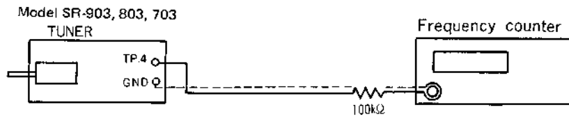
Fig. 21 FM MPX 19 kHz adjustment (Step. 1)
