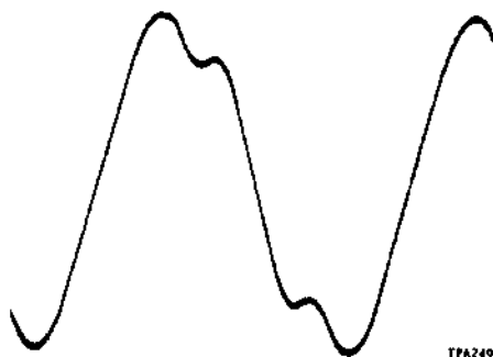
Fig. 2.2 1 kHz waveform with noise and distortion (The equivalent spectrum is shown below)
