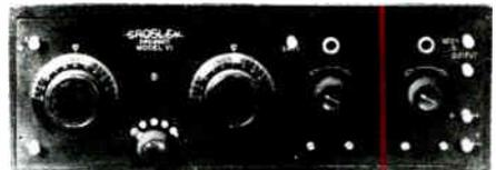
IN LATE 1923 THE MODEL VI WAS SOLD IN THE MORE COMMON CABINET WITH THE FAMILAR TUNING DIALS. INSIDE THE TRF CIRCUIT WAS UPDATED WITH THE SPIDERWEB-TYPE COILS INSTEAD OF THE DRUM TYPE. MOLDED RUBBER SOCKETS REPLACED PORCELAIN ONES, AND THERE WERE TWO LESS TAP SWITCH STOPS, ALL FOR \$30.
