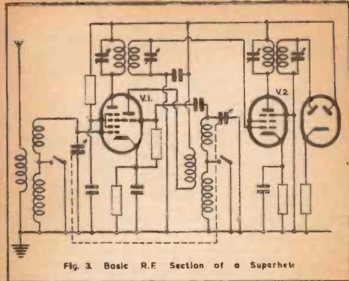
Fig. 3. Basic R.F. Section of a Superhet
