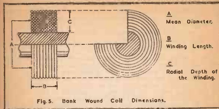
Fig. 5. Bank Wound Coil Dimensions.
