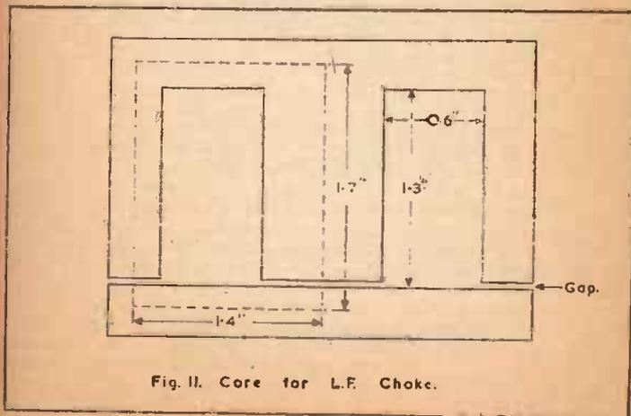
Fig. 11. Core for L.F. Choke.
