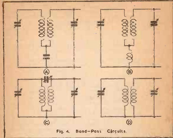
Fig. 4. Band-Pass Circuits.
