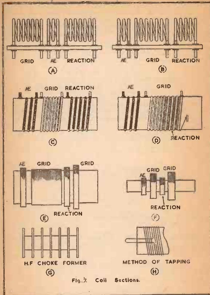
Fig. 7. Coil Sections.
