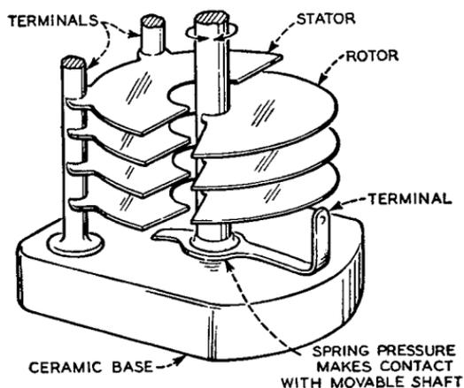
FIG. 31. Air capacitor.
