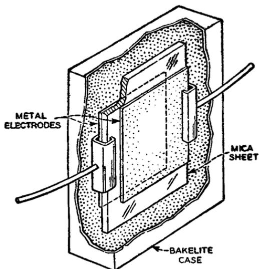
FIG. 27. Molded mica capacitor (enlarged).
