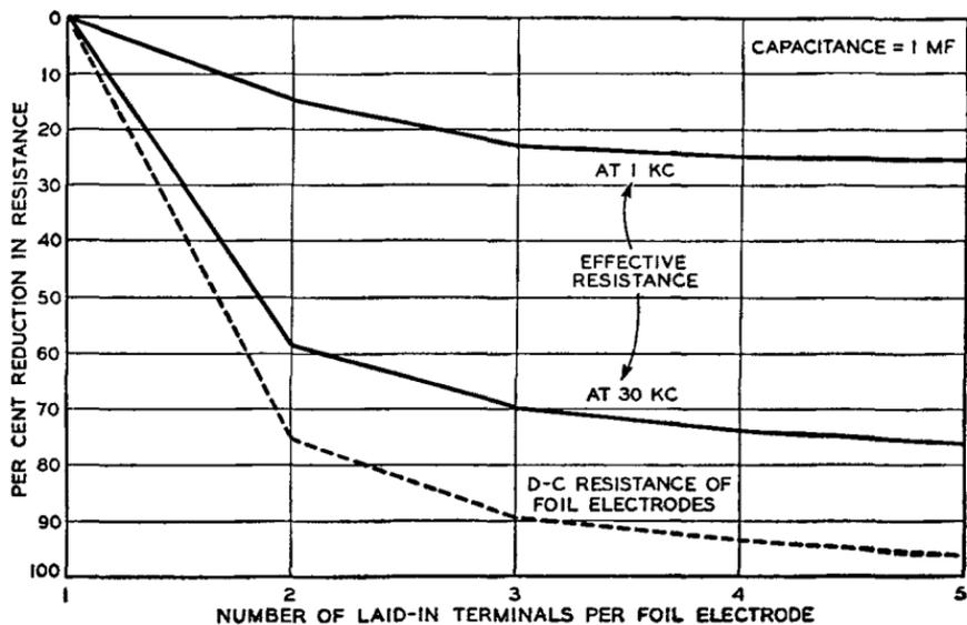
FIG. 10. Effective resistance is reduced by adding terminals, especially at higher frequencies.
