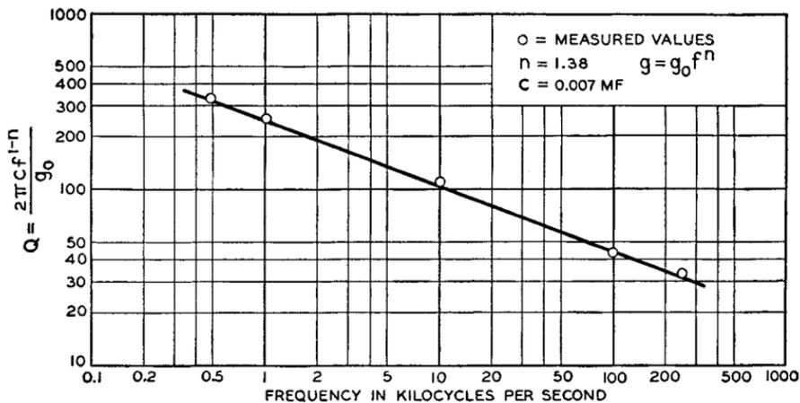
FIG. 12.  $Q$  versus frequency for tubular mineral-oil paper capacitor with dielectric loss dominant.
