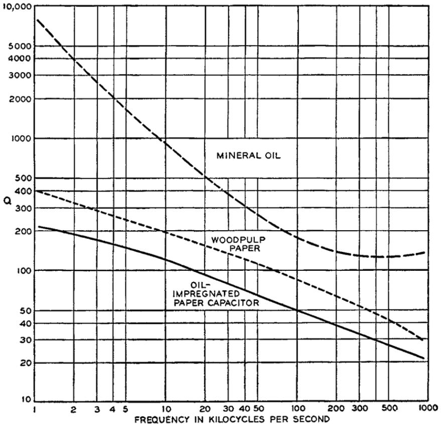
FIG. 24.  $Q$  versus frequency for mineral-oil paper capacitor. Shows limitation imposed by relatively poor  $Q$  of paper.
