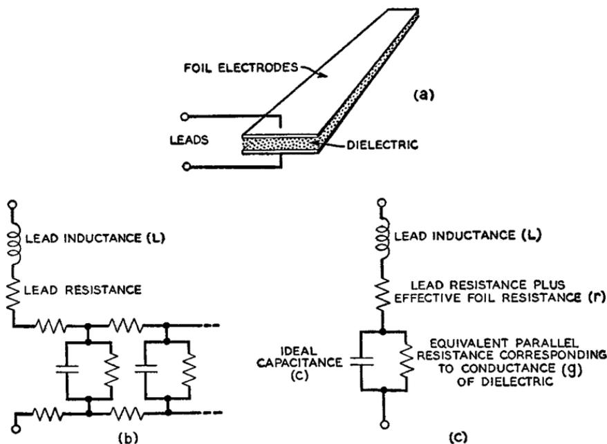
FIG. 5. Equivalent electrical circuit of a capacitor.
