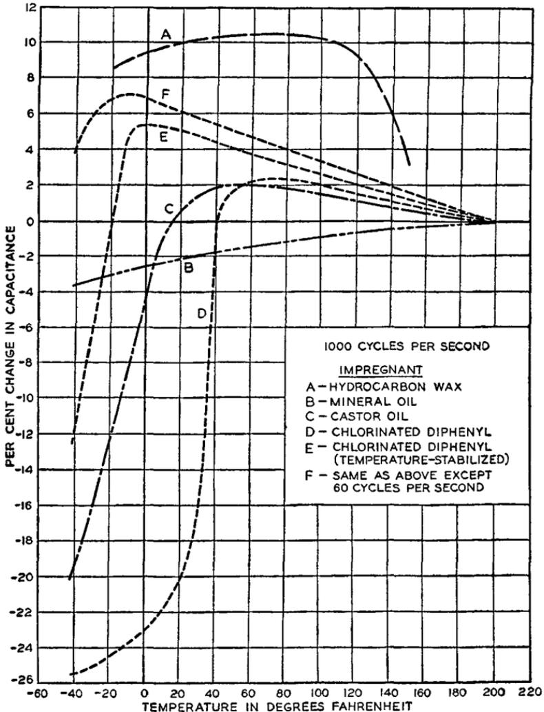
FIG. 25. Capacitance versus temperature for paper capacitors using commercial impregnants.
