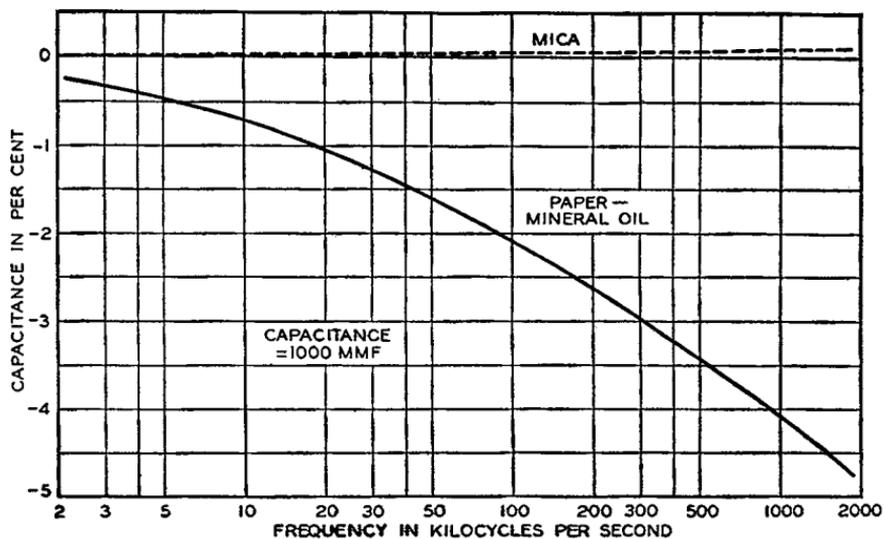
FIG. 28. Capacitance versus frequency for silvered mica and mineral-oil paper capacitors.
