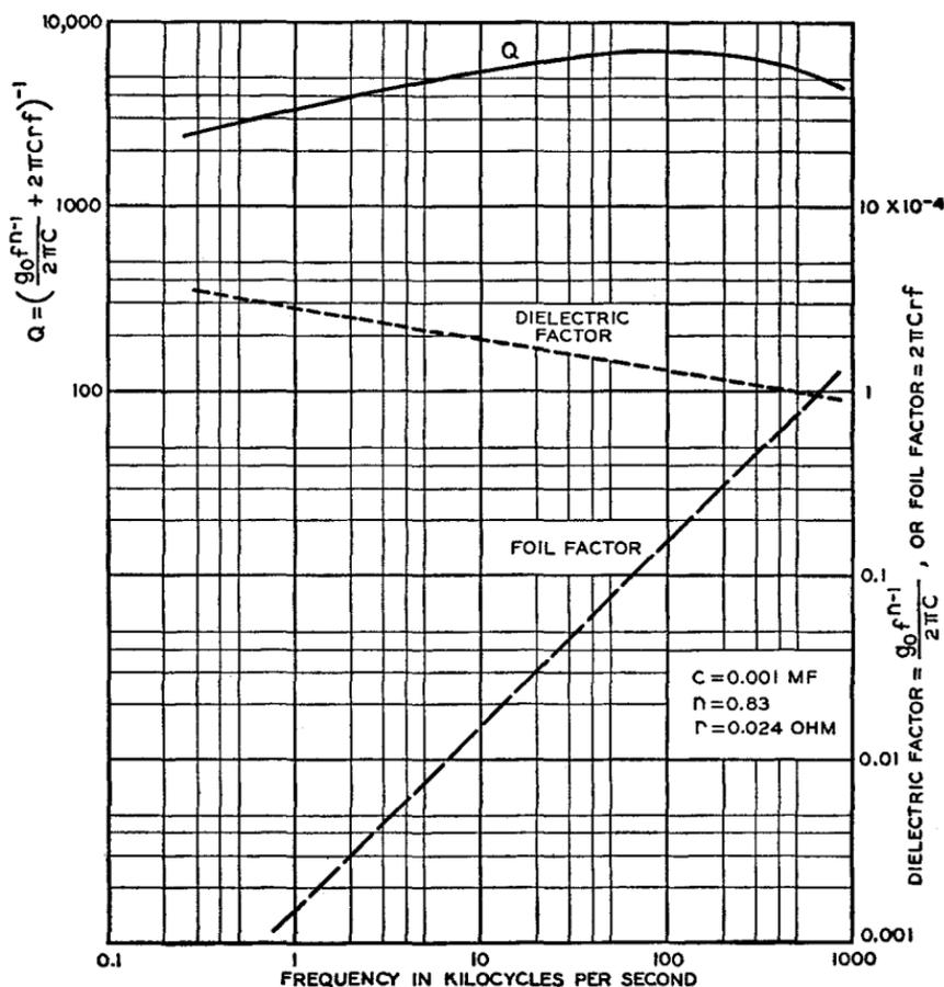
FIG. 14.  $Q$  versus frequency for silvered mica capacitor.
