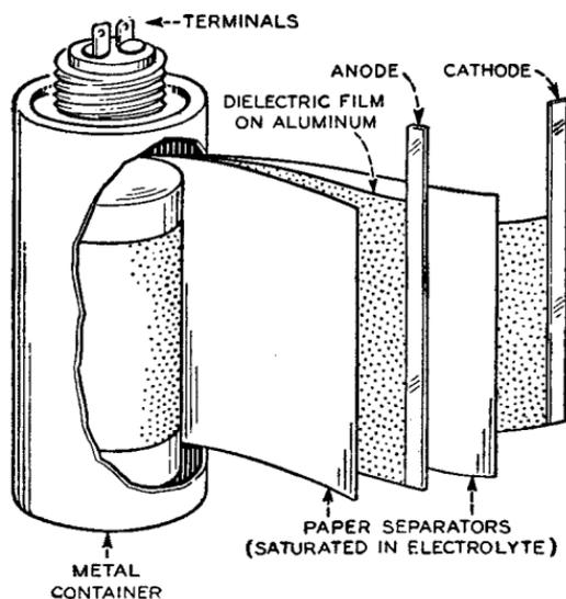
FIG. 20. Electrolytic capacitor.
