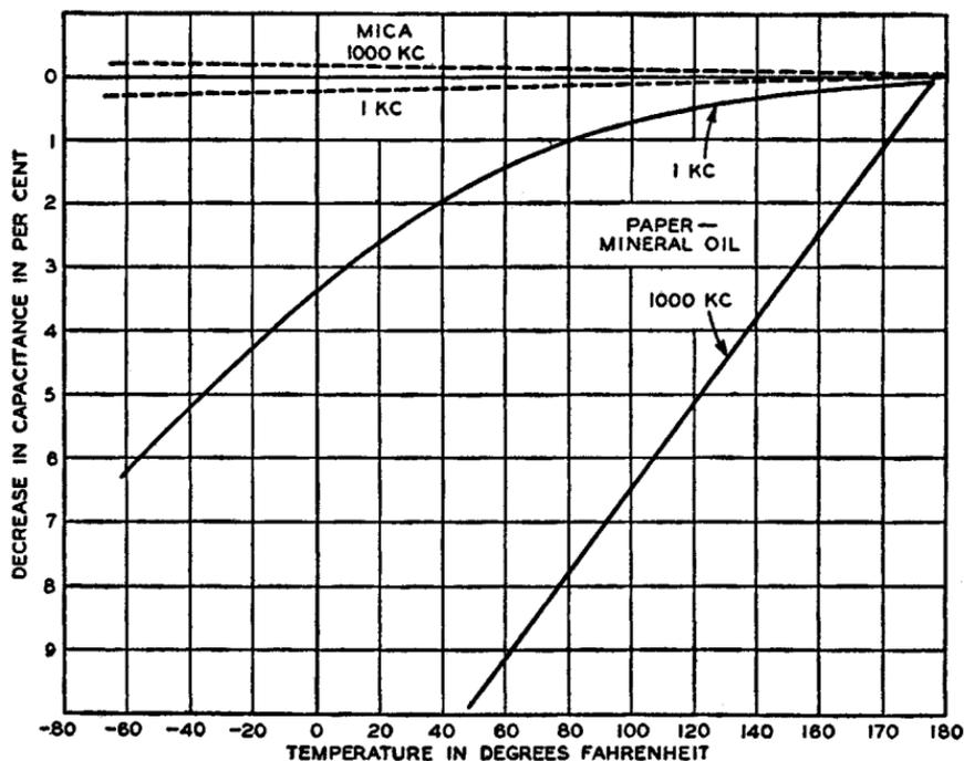
FIG. 29. Capacitance versus temperature for silvered mica and mineral-oil paper capacitors.
