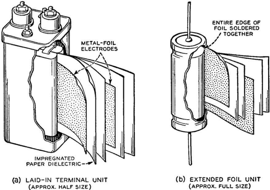
FIG. 22. Paper capacitors in hermetically sealed housings.
