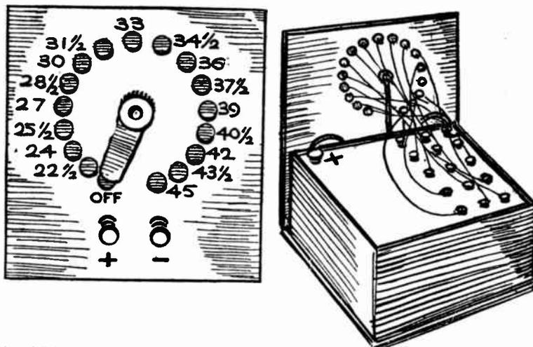
The "B" battery, which is the one made up of a lot of flashlight dry cells, should be mounted on a panel and each step of voltage should be wired to a switch contact point on the panel as shown. This enables you to make rapid and easy experiments with the amount of voltage you use and this often results in much stronger and clearer signals.
