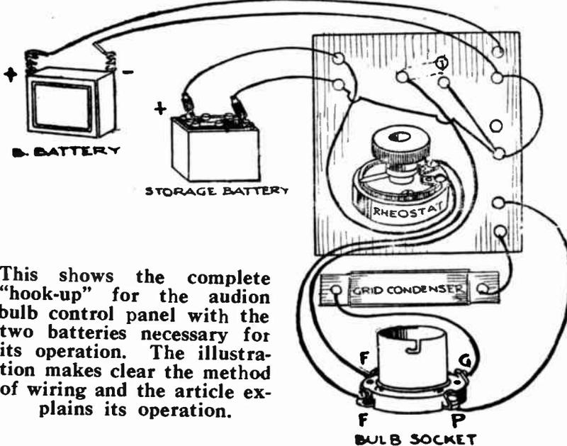
This shows the complete "hook-up" for the audion bulb control panel with the two batteries necessary for its operation. The illustration makes clear the method of wiring and the article explains its operation.
