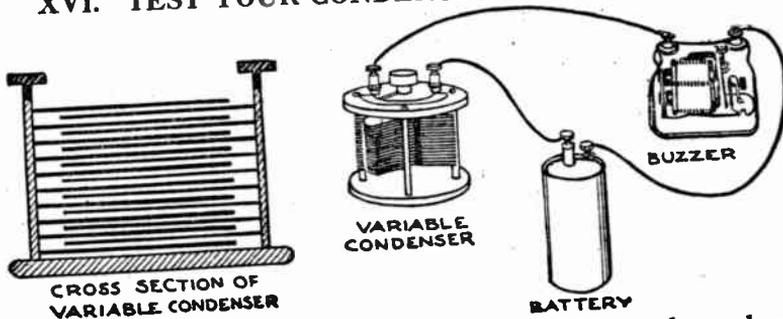
How to test a condenser. The left-hand diagram shows how the plates are arranged. There is no electrical connection between the two sets of plates. To the right is the hook-up for testing as explained in the article.
