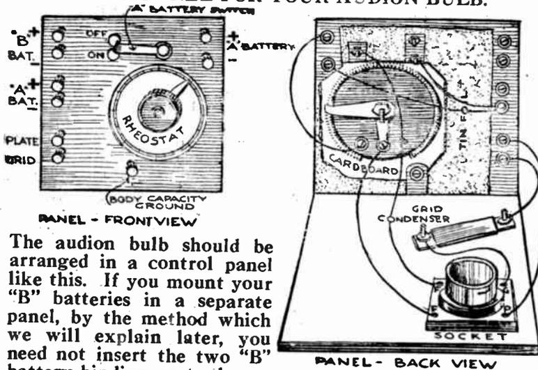
The audion bulb should be arranged in a control panel like this. If you mount your "B" batteries in a separate panel, by the method which we will explain later, you need not insert the two "B" battery binding posts shown, though it is better to do so.
