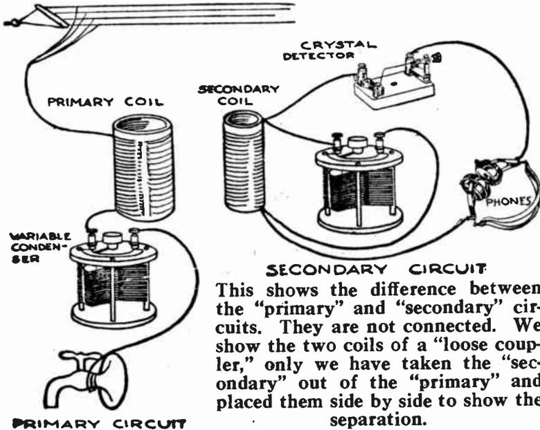
This shows the difference between the "primary" and "secondary" circuits. They are not connected. We show the two coils of a "loose coupler," only we have taken the "secondary" out of the "primary" and placed them side by side to show the separation.
