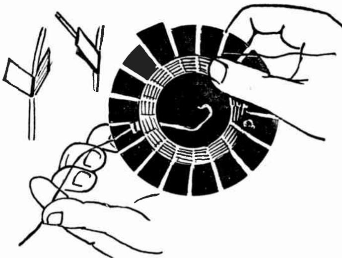
This is how a spider-web coil is wound and "tapped." For tapping, little pieces of thin brass or copper are best, cut as explained in the article. The upper sketches show how the metal strips are used.
