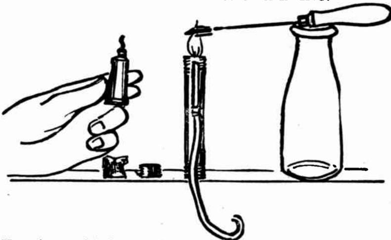
Here is a soldering outfit. The hand is holding a tube of "dope" or "salts"; under it is a piece of solder, next the cap that screws on the alcohol torch, next the torch itself and then the soldering iron resting on a milk bottle.
