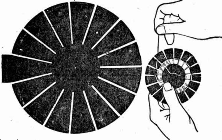
Here is a form that you can use for cutting out the cardboard to make spider-web coils. On the right, the picture shows the method of winding them.
