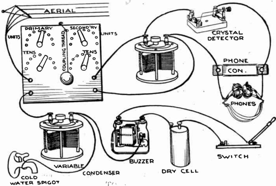
These are the simplest hook-ups for crystal and bulb detectors using the spider-web outfit described in this issue. But remember that, if you use variable condensers, you do not need the "units" taps on your spider webs.
