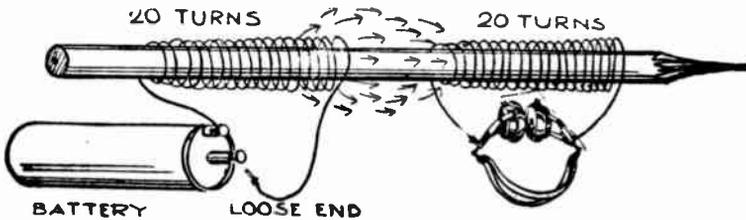
Here we have a complete sending and receiving set in its very simplest form and also an excellent illustration of what an induction coil, a loose coupler and "coupling" mean. The article explains it.
