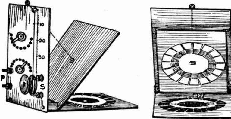
Here is a handily made little unit for mounting two spider-web coils to make a coupler. The upper pictures are actual views of such a unit. The lower one is a diagram of the panel arrangement.
