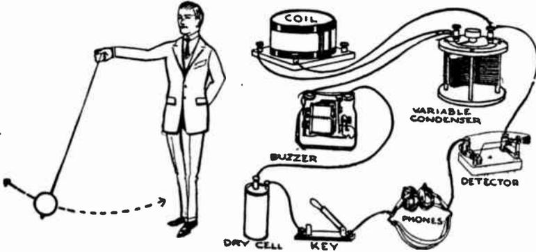
A radio circuit vibrates or swings back and forth just as a pendulum does. The longer the pendulum, the longer arc it makes, and the greater length of time it takes to make a vibration. To the right is a collection of instruments that make vibrations and detect them in a radio circuit. We have means of varying them just as we vary the vibrations of the pendulum. The article explains it.
