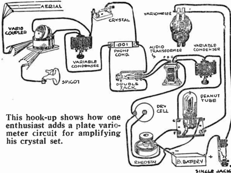
This hook-up shows how one enthusiast adds a plate variometer circuit for amplifying his crystal set.
