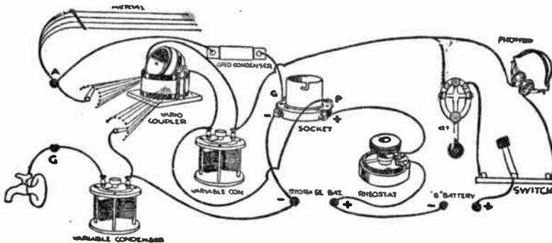
**This hook-up shows how to turn your single circuit regenerative receiving set into a low-powered transmitting set for using continuous waves**
