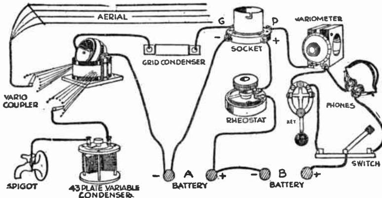
By means of this hook-up and the instructions given in the accompanying article a double circuit set with one or two variometers may be changed into a fairly satisfactory transmitting set for continuous wave signals
