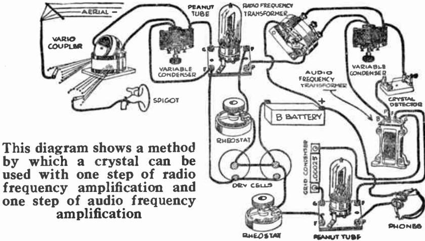
This diagram shows a method by which a crystal can be used with one step of radio frequency amplification and one step of audio frequency amplification
