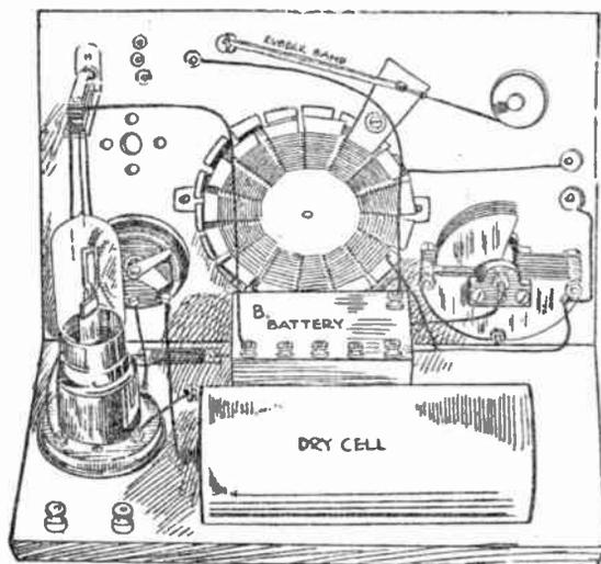
These illustrations show the method by which the \$15 bulb set was mounted for operation
