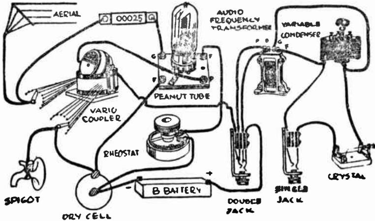
Here is an interesting hook-up for inserting a "single-circuit regenerative" set ahead of the crystal detector
