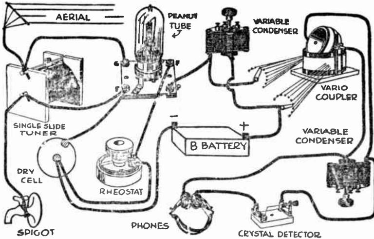
This diagram shows the best method of adding tuned plate radio frequency amplification ahead of a crystal detector
