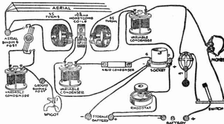
By means of this diagram and three smaller size coils, the regular three honeycomb coil receiving hook-up can be transformed into a fairly efficient and satisfactory sending set for continuous waves
