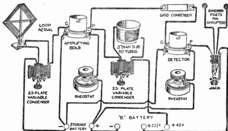
Here is a very efficient hook-up for two bulbs and a loop aerial, the circuit using one stage of radio frequency amplification by the tuned plate method
