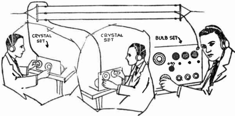
By this hook-up of a three-wire aerial, two men with crystal sets can hear distant stations re-radiated from the bulb set that uses the central wire
