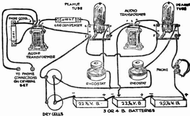
**This hook-up shows a two-stage amplifying outfit that can be added to any crystal set**
