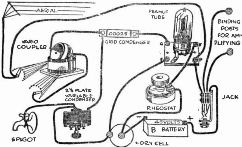
This arrangement shows a very efficient use of a variocoupler in the Gibbons hook-up
