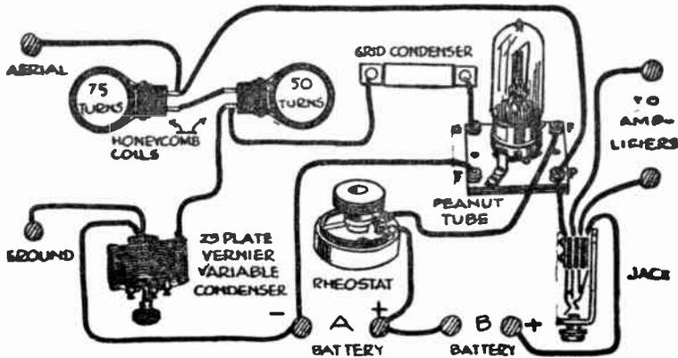
**It would be hard to get a more efficient radio hook-up than this adaptation of the Gibbons arrangement, using two honeycomb coils for tuning**
