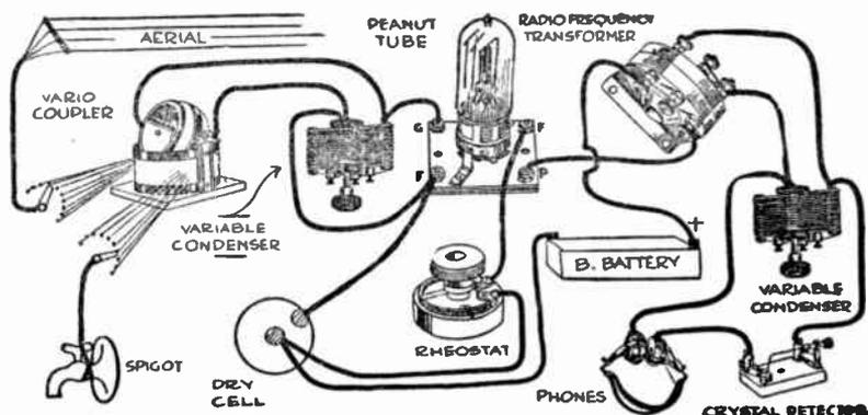
**This hook-up shows how to use the peanut tube with one step of radio frequency amplification ahead of the crystal detector**
