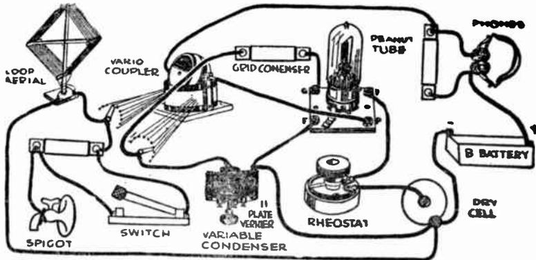
This diagram shows an interesting hook-up by which a loop aerial and a variocoupler can be used with a ground connection
