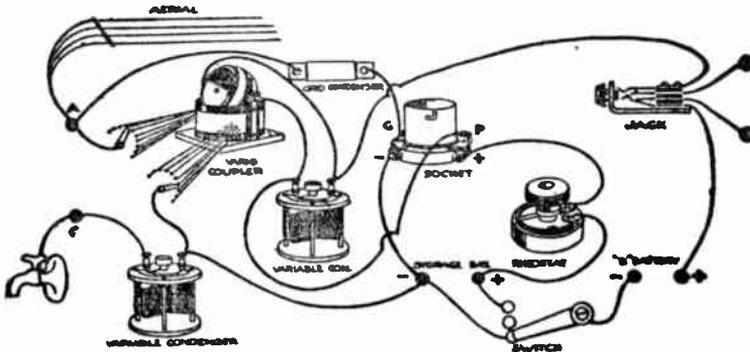
The addition of a twenty-three-plate variable condenser as shown in this hook-up gives much finer tuning to the single-circuit regenerative set
