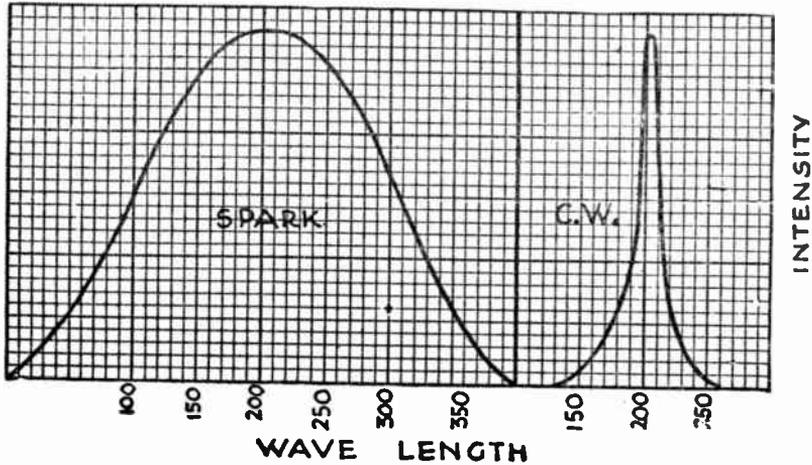
These two curves show the difference in intensity between signals sent out by the spark method and by the C. W. method and show also how broad the spark signal is and how sharp the C. W. signal is
