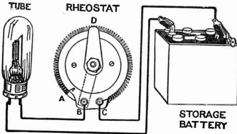
The flow of electrons in the tube is governed by the amount of resistance included in the rheostat from the storage battery. The current passes from the storage battery to C then around the resistance winding to D and so down to B and to the bulb. As the blade is moved the amount of resistance wire between C and D is varied, and thus the flow of electrons is controlled as explained in the accompanying article
