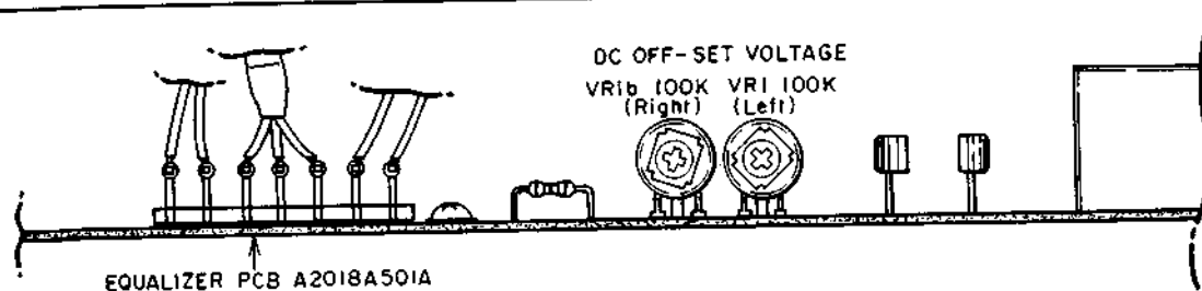
Fig. 8 Equalizer P.C Board A2018A501A
