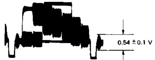
Fig. 5-34 NTSC playback burst level
