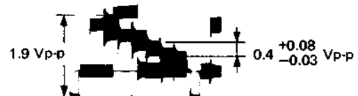
Fig. 5-31 SECAM playback color level
