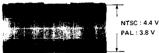
Fig. 5-23 Recording FM level
