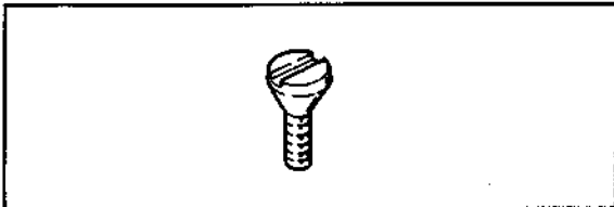
Fig. 7-11 Head dihedral adjust screw
